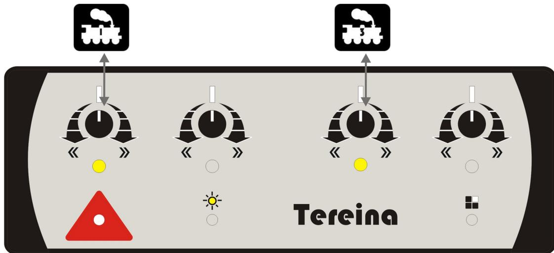
Figure 2.2: Example of controlling locomotives by 1st and 3rd knobs
