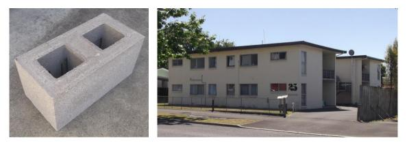
Figure 5.1: A typical hollow brick used in the construction of apartment blocks in New Zealand, and an example of a ten-unit apartment block<sup>26</sup> (Source: Author)
