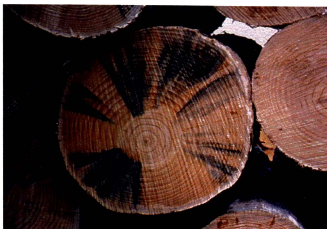
Figure 1.5: Discolouration on unseasoned timber caused by a sapstain fungus (Photo courtesy of Forest Research).
