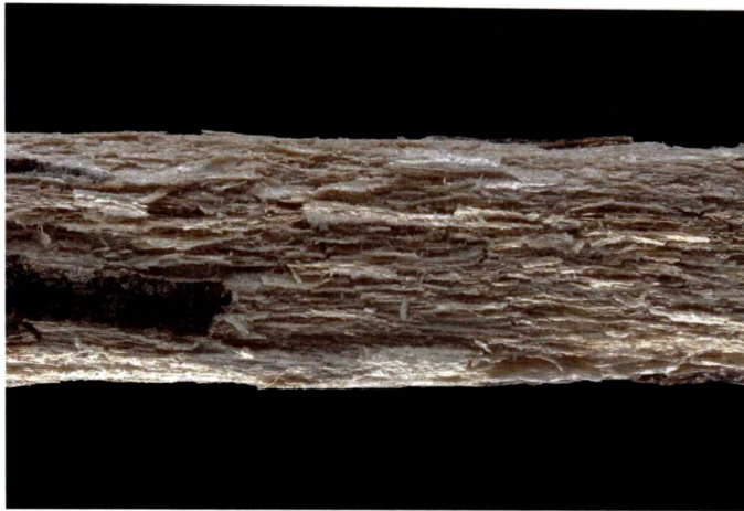
Figure 1.3: Damage caused by a white rot decay fungus on untreated timber (Photo by John Barran).
