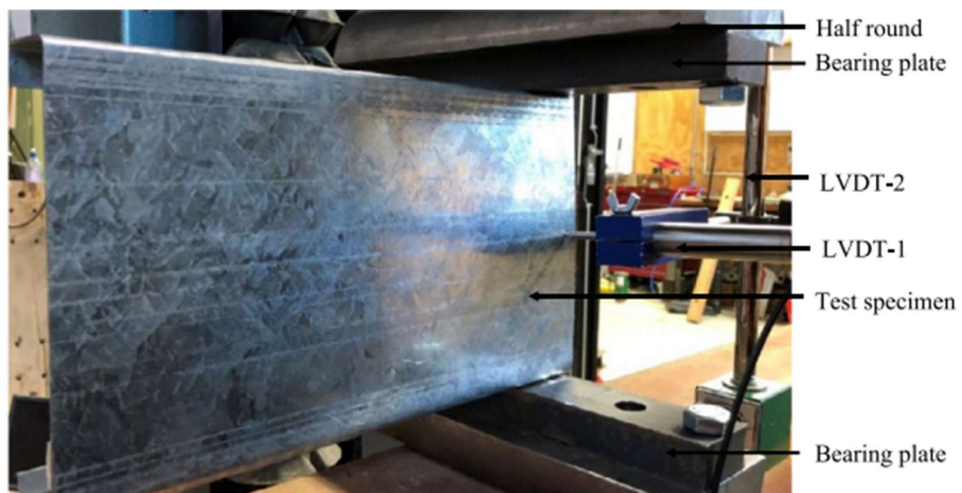
b. End-two-flange (ETF) loading conditions
