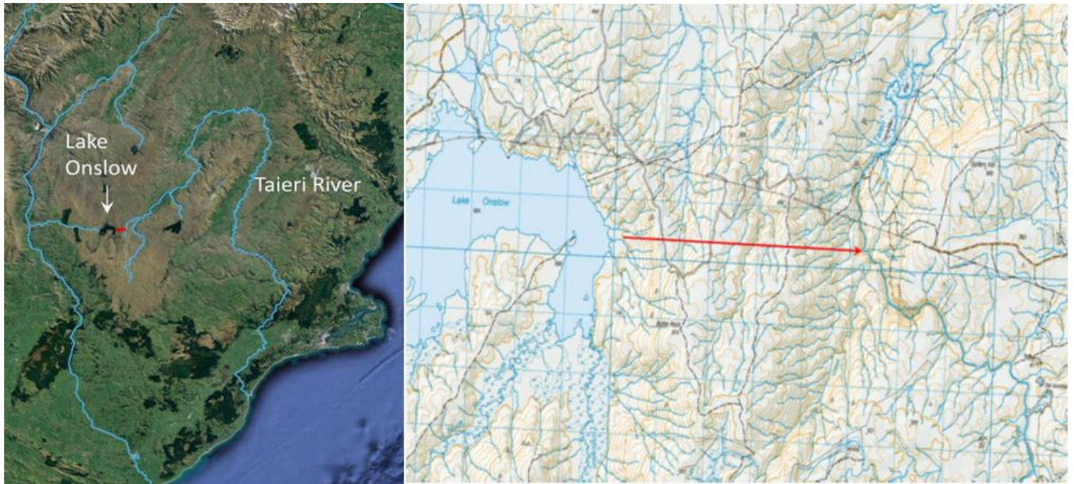
Figure 5.9. Possible tunnel connection (red) at 720 m elevation between a future expanded Lake Onslow and the Riddles Creek Taieri headwater, which flows into the upper Taieri River via Bonds Stream (Figure 5.10).
