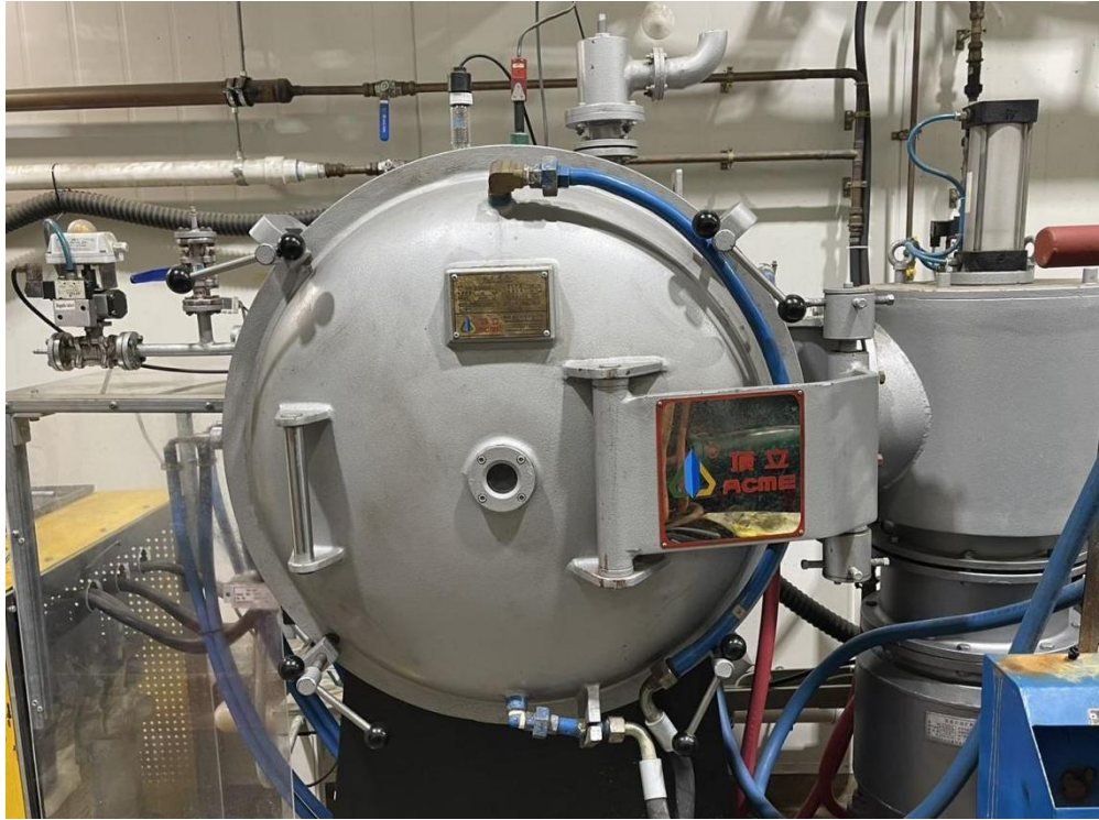
Fig 3.10 Vacuum sintering furnace
