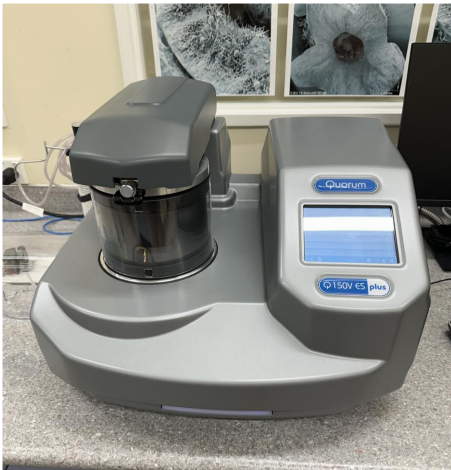
Figure 20 Sputter Coating equipment
