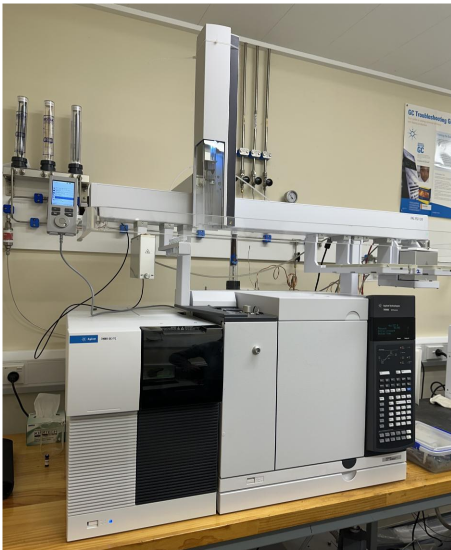
Figure 9 Agilent model 7890B GC with PAL auto-sampler and MS Triple quad.
