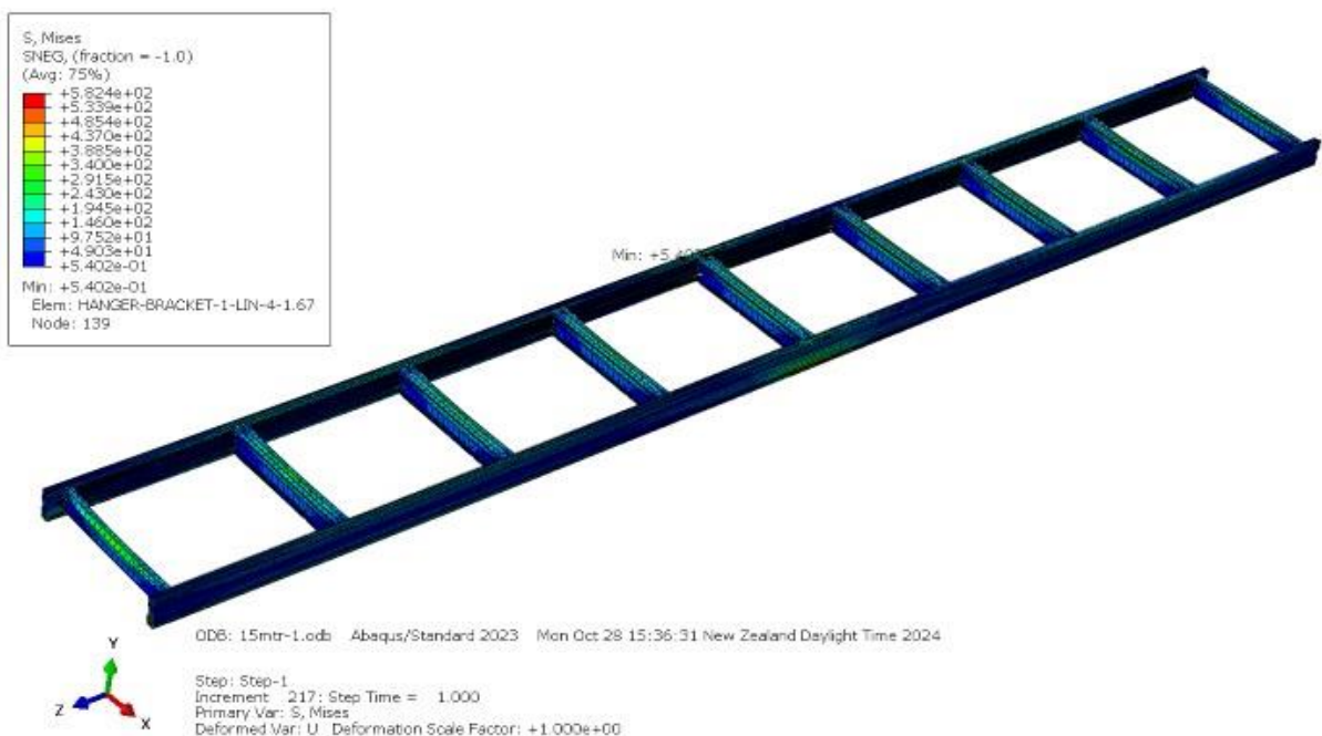
Figure 86 shows Results from the Von Mises stress analysis of CFS foot bridge.
