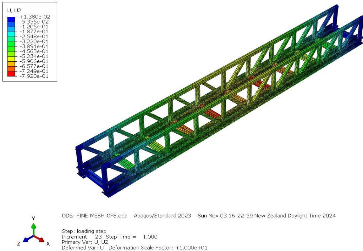
Figure 34 shows final deflection of bridge.
