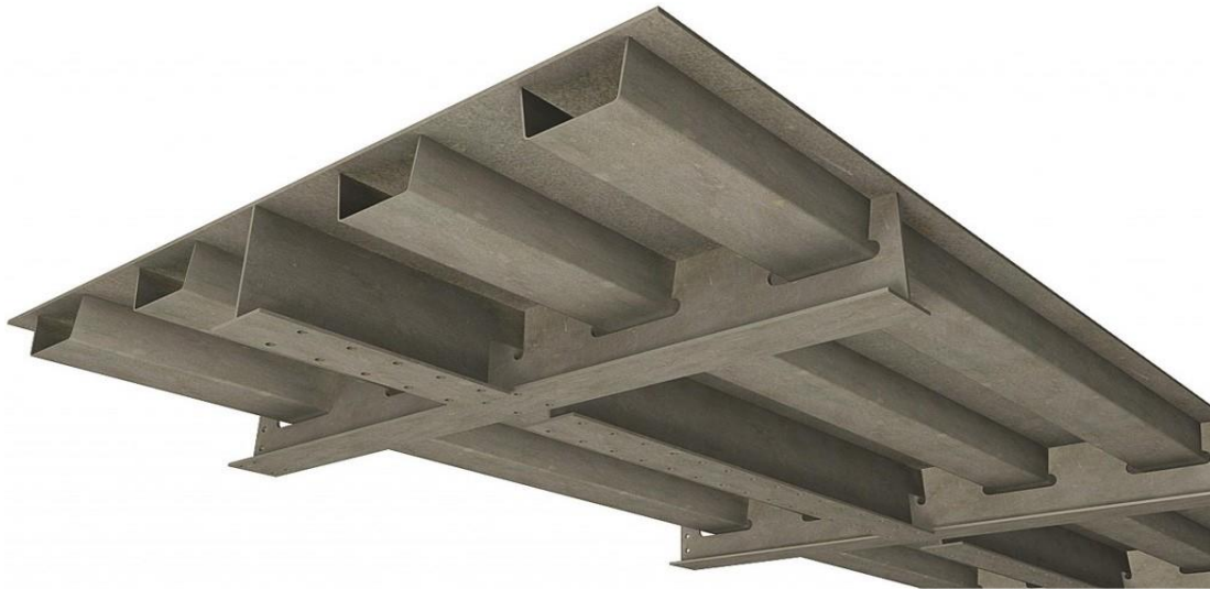
Figure 74 shows steel orthotropic decks [65].
