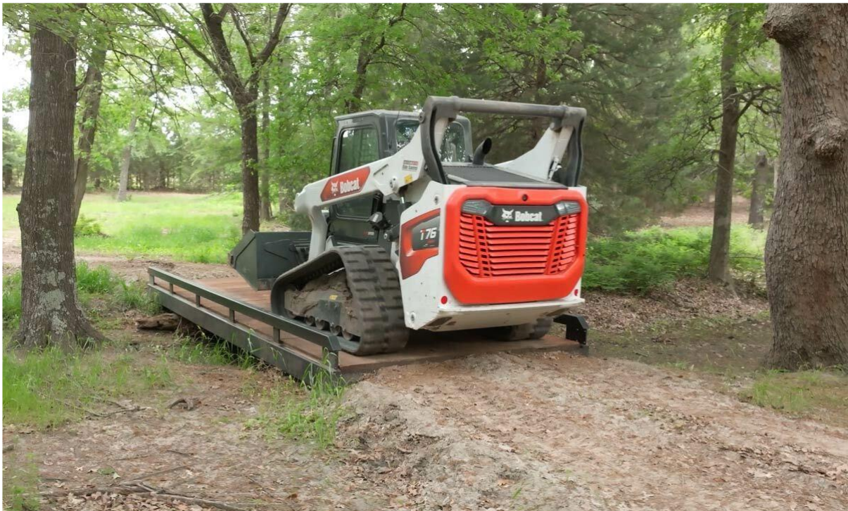
Figure 76 shows flat bridge used as utility bridge [67].
