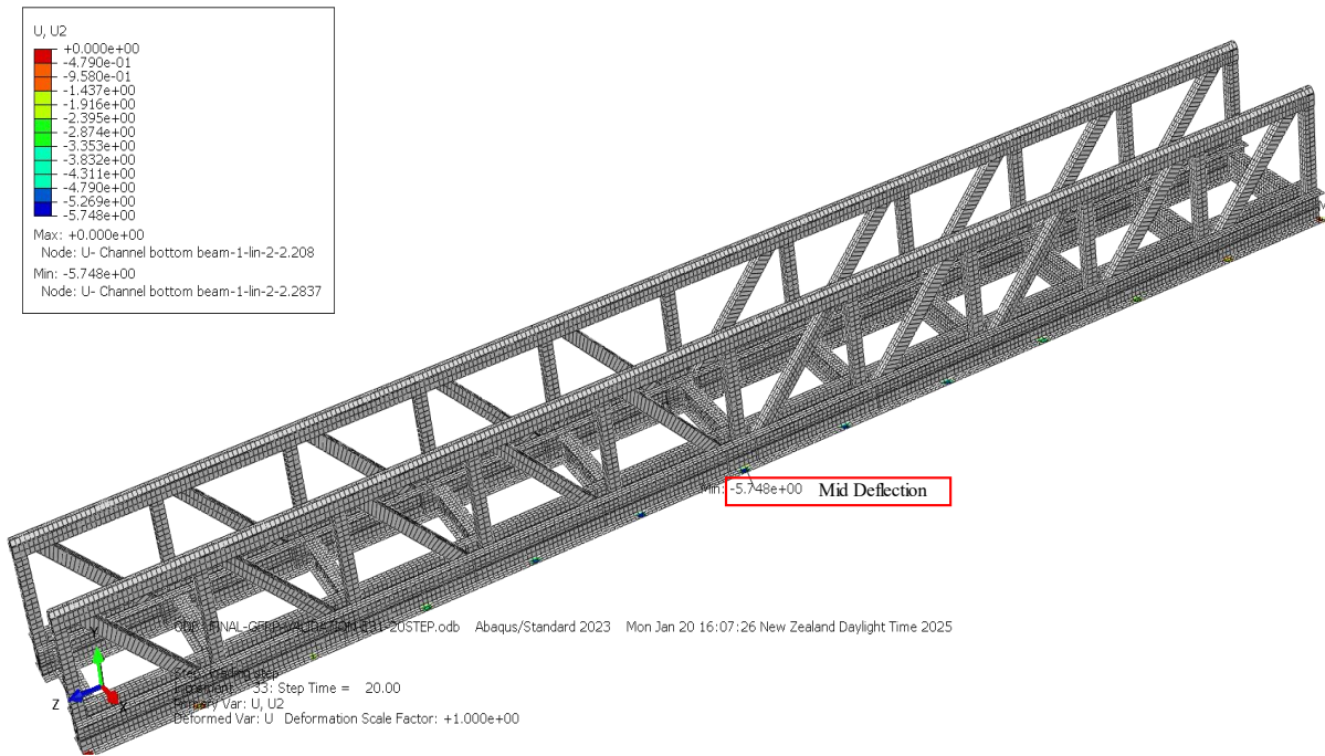
Figure 27 Mid span Deflection for validating model [54].
