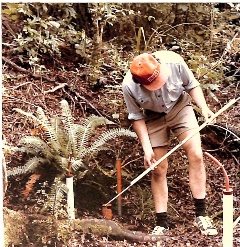
Plate 4.7 : Saturated soil moisture conditions were measured with narrow bore piezometers (orange). Observations were made of the weekly peak water table elevations and the water table elevations at the time of observation. The P.V.C. tubes are vacuum lysimeters used by Phipps (1982)
