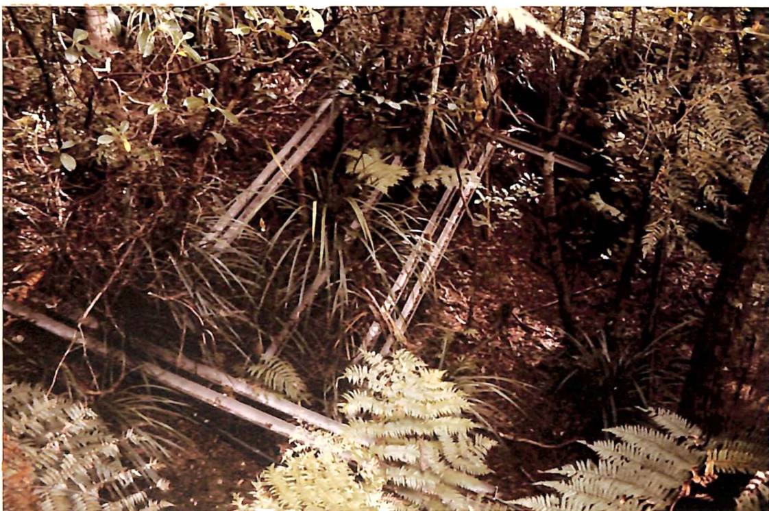
Plate 4.3 : The forest interception plot showing the arrangement of the collecting troughs. Throughfall from these troughs was bulked into a single recording device
