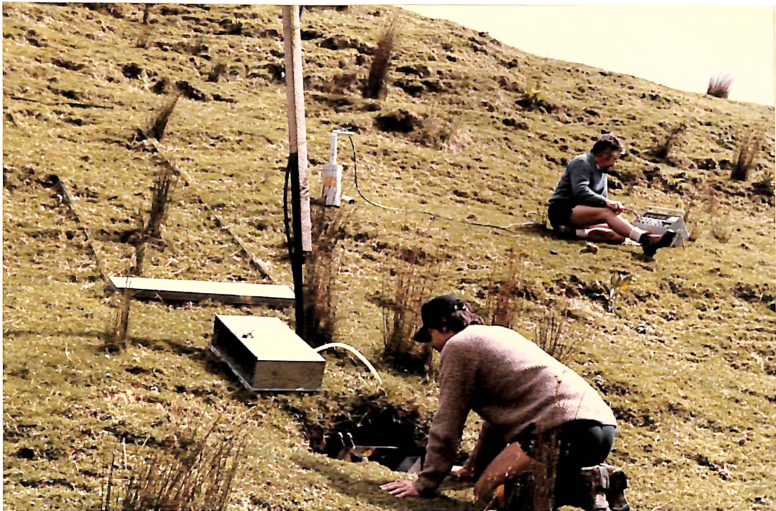
Plate 4.4 : The arrangement of a surface runoff plot and soil moisture sampling site. Note the tipping bucket for recording surface runoff continuously
