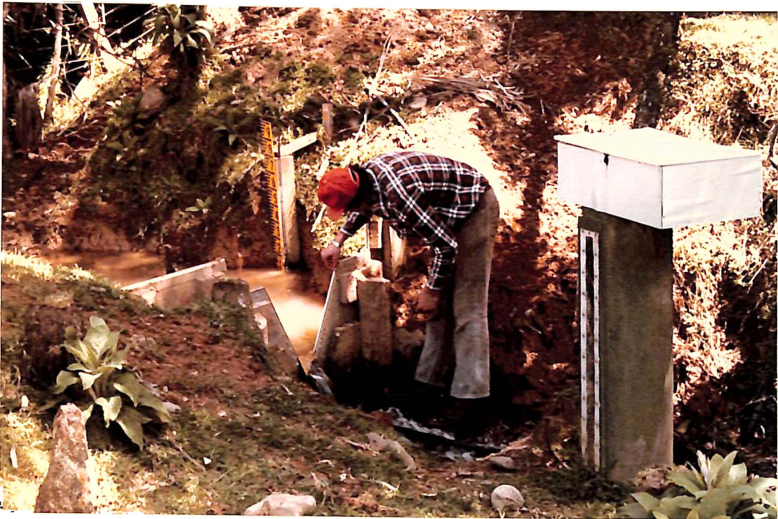
Plate 4.2 : The weir site at the outfall of the forest catchment showing the 'V' notch and rectangular addition
