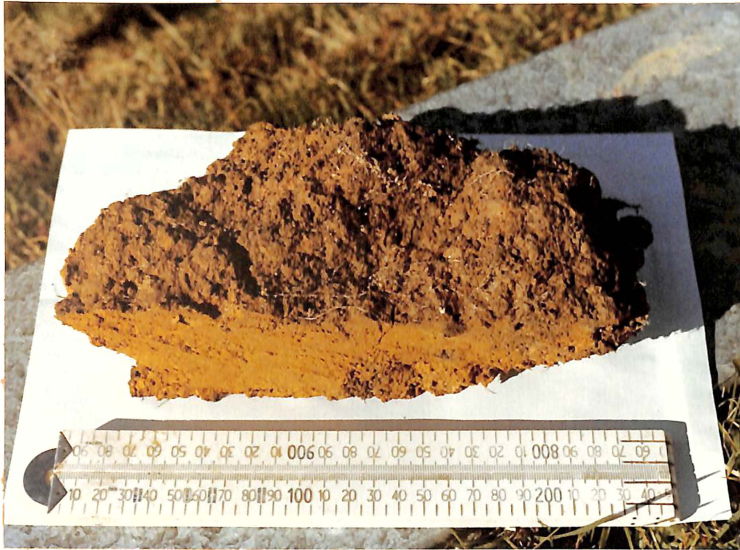
Plate 6.3 : The soil prism that was removed to show the features in plate 6.2. Note the roots and organic coatings on the prism surface
