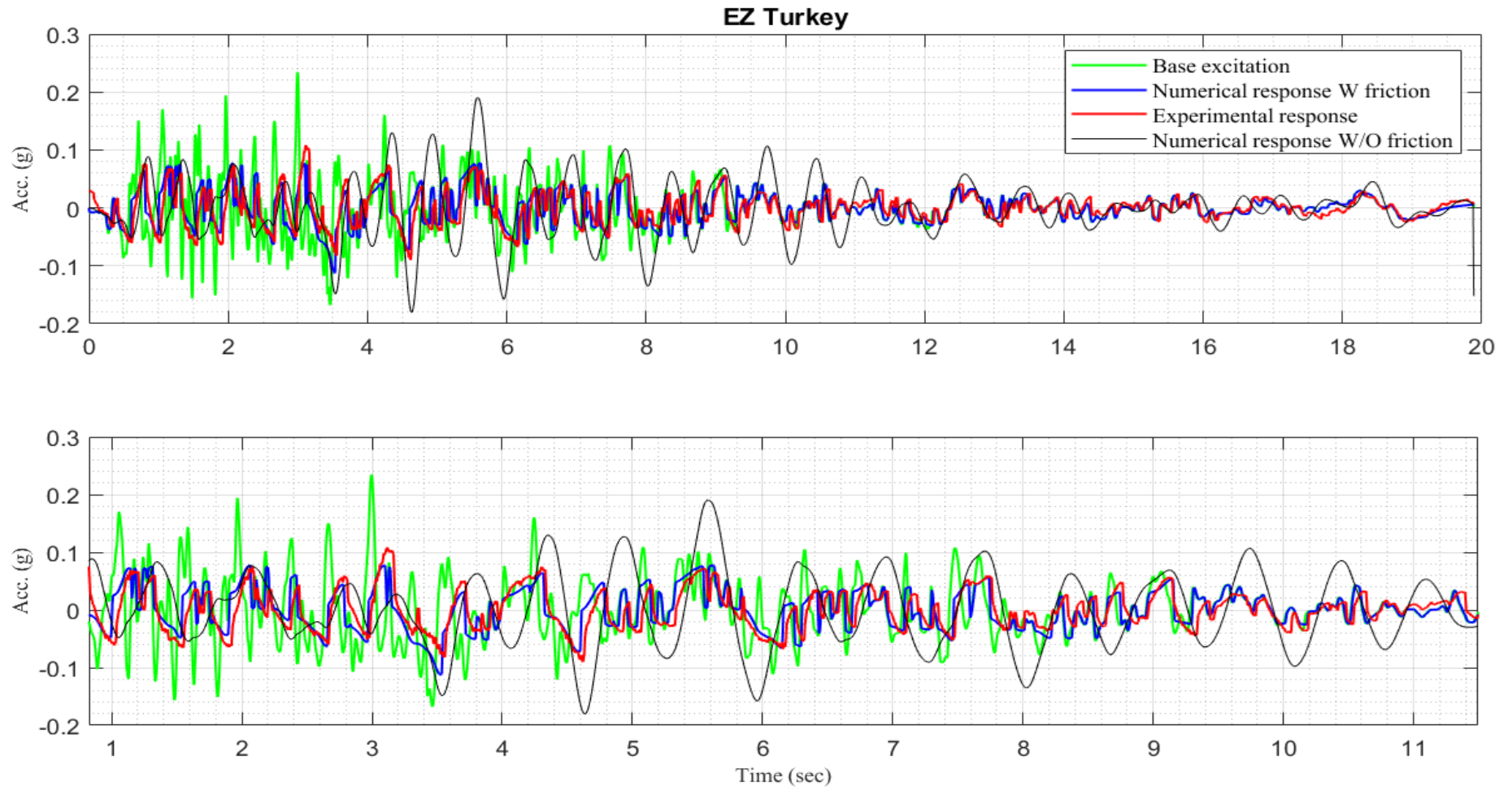
Figure 5.13. EZ Turkey base excitation, experimental and numerical response acceleration time histories for the mechanism with m = 0.708 kg, l = 0.1 m, k_h = 280 N/m, k_v = 140 N/m and \theta_0 = 30^\circ .
