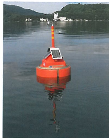
Figure 2. LERNZ High frequency monitoring buoy. Photo: Chris McBride.
