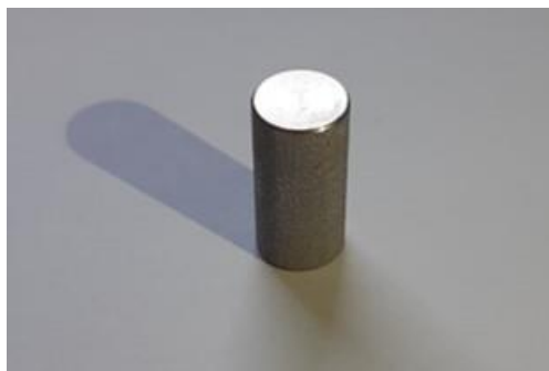
Figure 2.5: Compression sample with machined ends. Approx. 10 mm diameter, 20 mm long.
