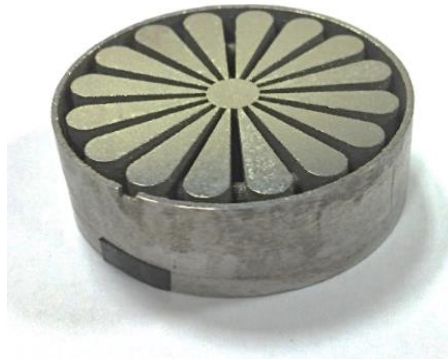
Figure 2.7: Segmented disk for microstructure and hardness investigation.
