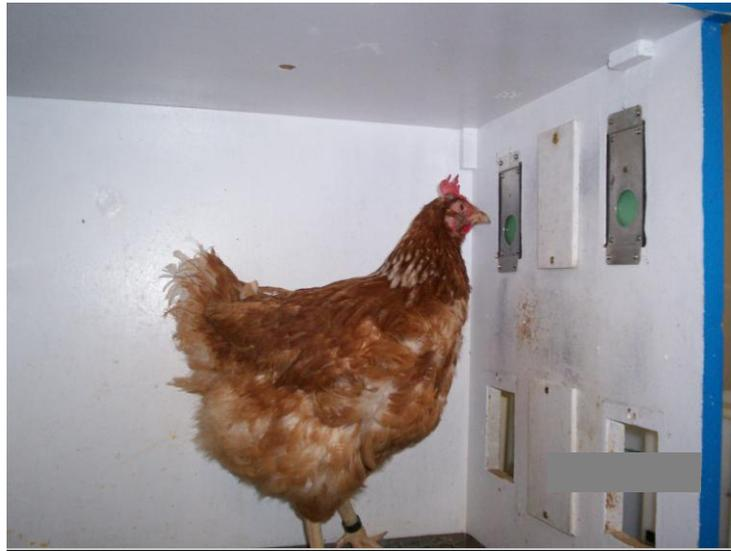
*Figure 22.* The experimental chamber with two response keys which lighted green when in effect, two food magazines directly below the keys delivered wheat, puffed wheat or both based on experimental conditions
