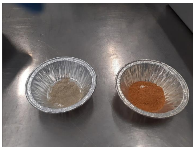
Figure 2.14. Comparison of sediment before and after being taken to the muffle furnace
