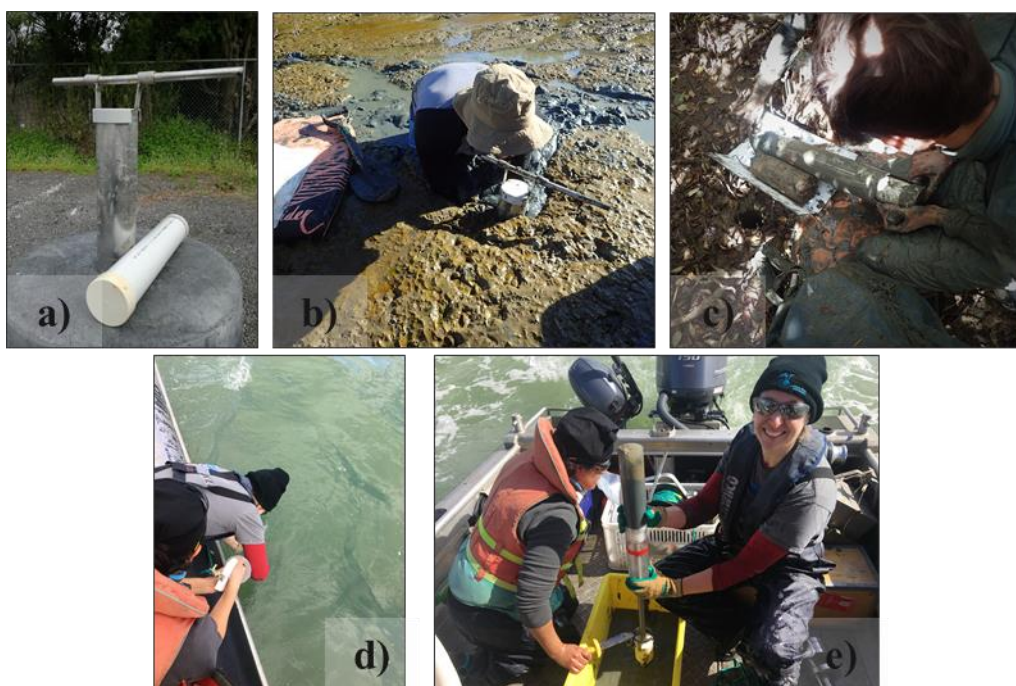
Figure 2.4. Corers used in field sampling. a) Push corer with handle to generate pressure and torsion. b) Push corer in a mudflat station. c) Land core extraction. d) Boat sampling. e) Core extraction from the gravity corer
