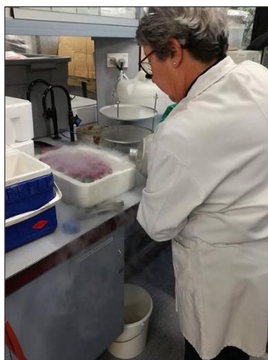
Figure 2.12. Samples are treated with liquid Nitrogen prior to freeze dry treatment.
