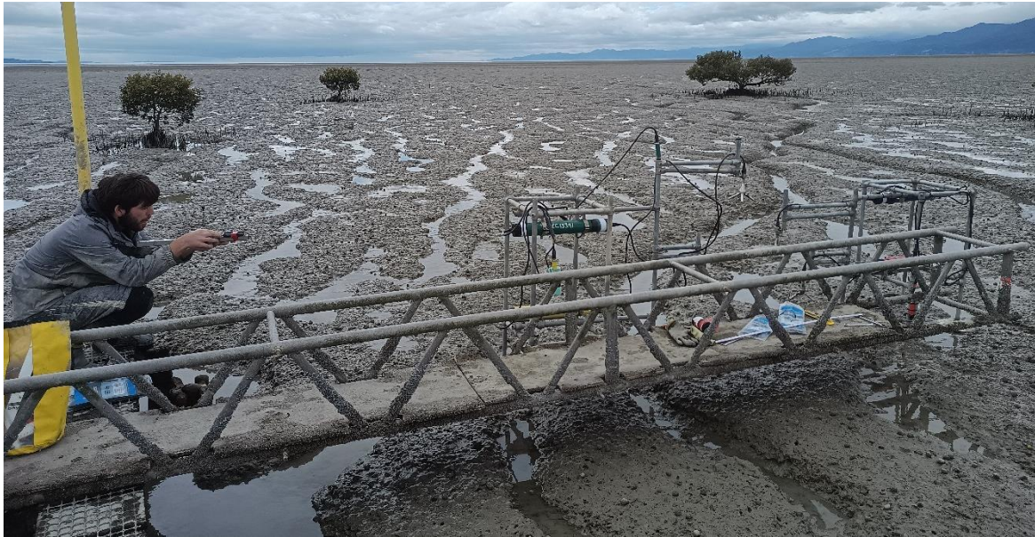
Figure 2.4: Cantilevered platform extending out perpendicular to the shore normal orientated boardwalk. Instruments were deployed from the platform to minimise disturbance to the substrate. During measurement the platform was retracted to prevent any disturbances to flow.
