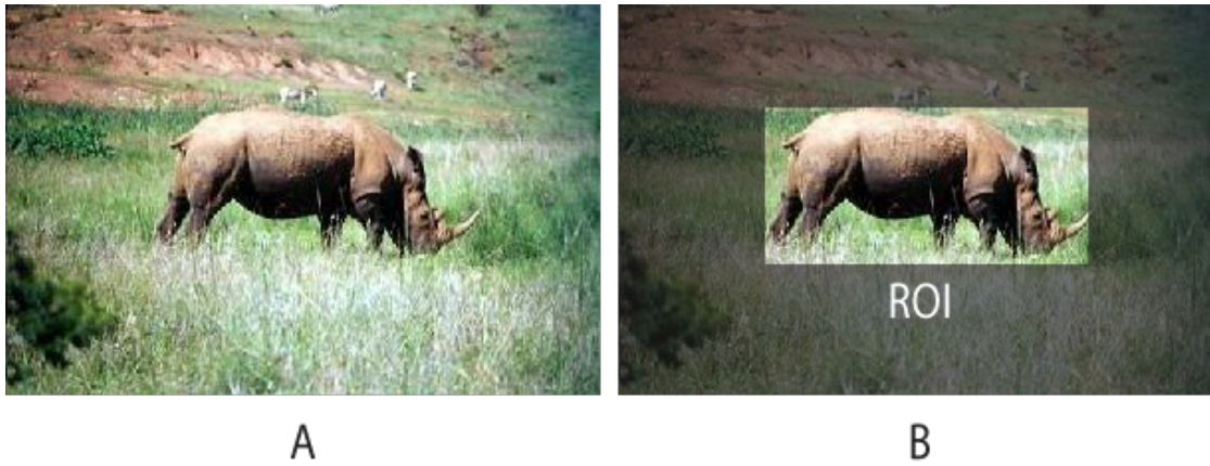
Figure 6.1: The entire image is used to extract visual features in A. In B, only the ROI is used to extract visual features.
