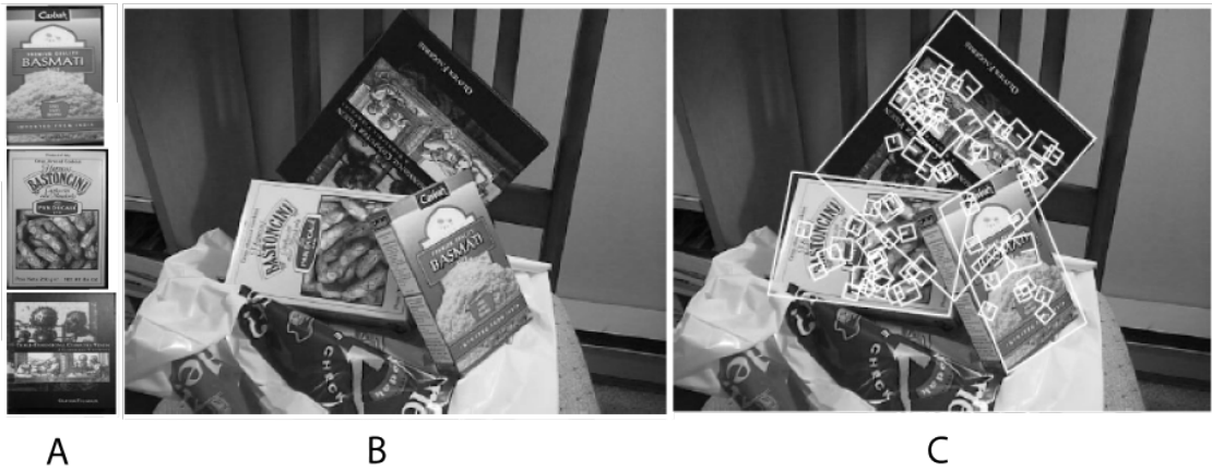
Figure 2.3: Model images of planar object are shown in A: Testing image is shown in B: Recognition results are shown in C with keypoint matches. [90]
