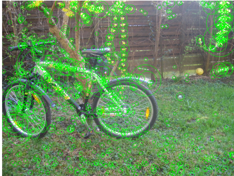
Figure 3.2: Keypoints (green eclipses) are detected on the image. The scale of the keypoints is not fixed.
