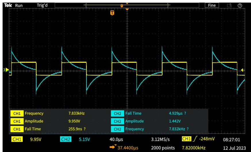
Figure 5.6: The oscilloscope output displays the square gate voltage (yellow) and the filtered output (blue). The high-pass filter, designed with a cutoff frequency of 1 kHz, is tested using a higher frequency input to demonstrate its filtering capabilities.
