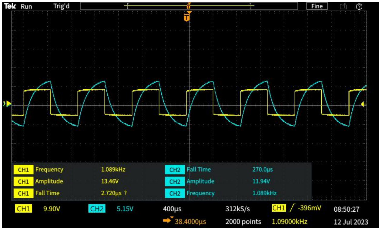
Figure 5.3: The oscilloscope output displays the square gate voltage (yellow) and the filtered output (blue). The low-pass filter, designed with a cutoff frequency of 800 Hz, is tested using a medium-range frequency input to demonstrate its filtering capabilities.
