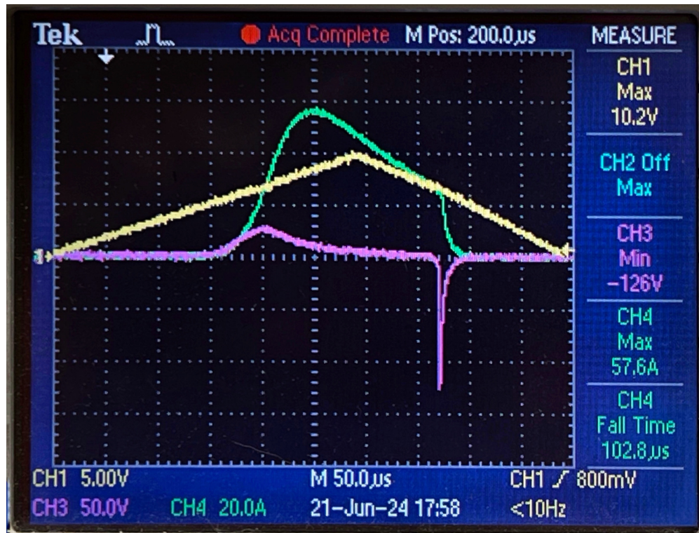
Figure 7.5: This figure demonstrates the cTBS pulse generated by the MATLAB model with a 500 \mu\text{s} pulse width, shown with the experimental test setup. Yellow represents the gate voltage, green depicts the TMS current pulse, and magenta illustrates the TMS voltage pulse in the experimental setup.
