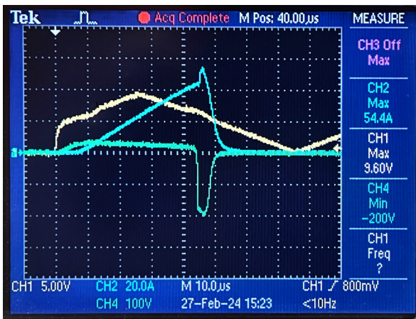
Fig. 10: Oscilloscope measurement of 50% triangular gate voltage (yellow), TMS coil current measured using Tektronix A622 (blue), voltage across the TMS coil (green)
