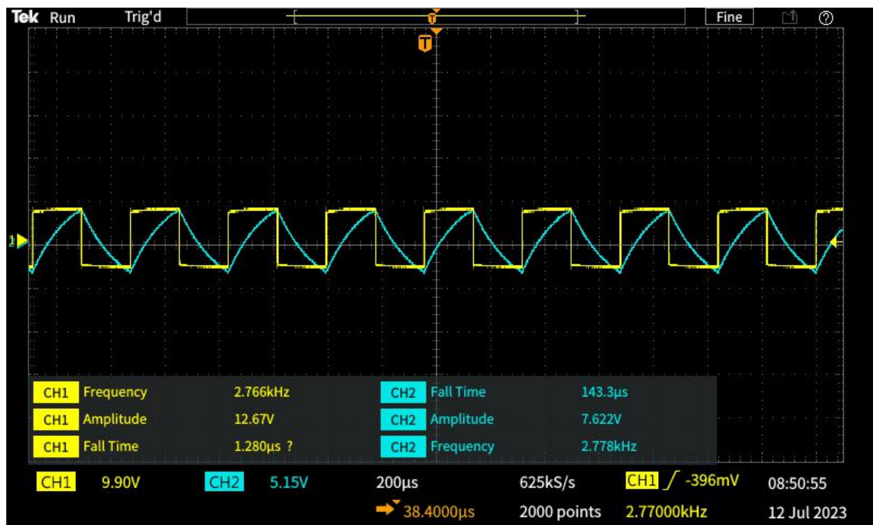
Figure 5.4: The oscilloscope output illustrates the square gate voltage (yellow) alongside the filtered output (blue). Designed with a cutoff frequency of 800 Hz, the low-pass filter is tested using a higher frequency input, effectively demonstrating its filtering capabilities.
