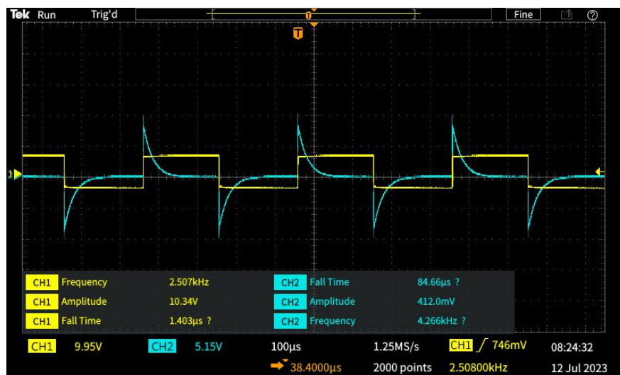
Figure 5.7: The oscilloscope output displays the square gate voltage (yellow) and the filtered output (blue). The high-pass filter, designed with a cutoff frequency of 1 kHz, is tested using a medium-range frequency input to demonstrate its filtering capabilities.
