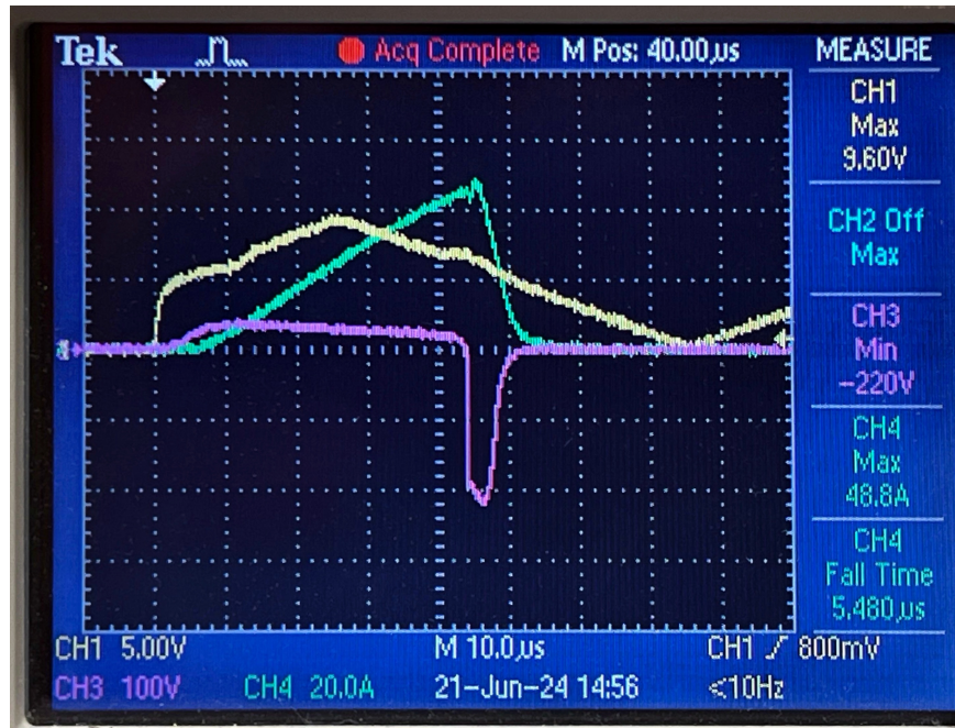
Figure 7.4: Oscilloscope capture of a single pulse within the cTBS pattern shown in Fig. 7.2, providing enhanced illustration and clarity of the pulse characteristics. Yellow represents the gate voltage, green depicts the TMS current pulse, and magenta illustrates the TMS voltage pulse in the experimental setup.
