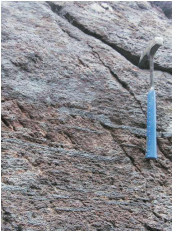
Figure 2.18: Strongly welded facies at site 20. Faint clast outlines are visible in the face as stretched ribbons. Hammer handle measures 30cm.
