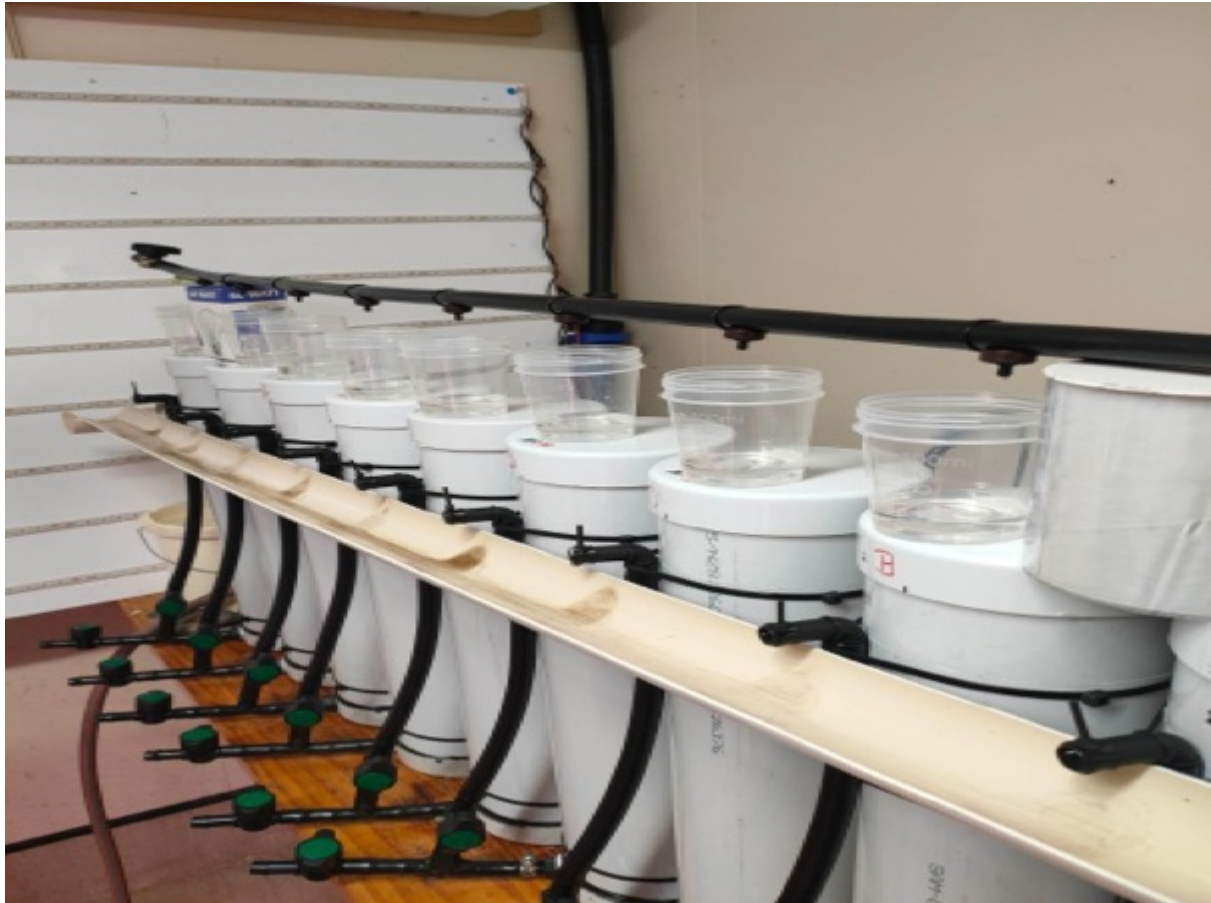
Figure 4. Stream water collecting in measuring cups (100 mL) placed underneath dripper for 1 minute to measure flow rate.
