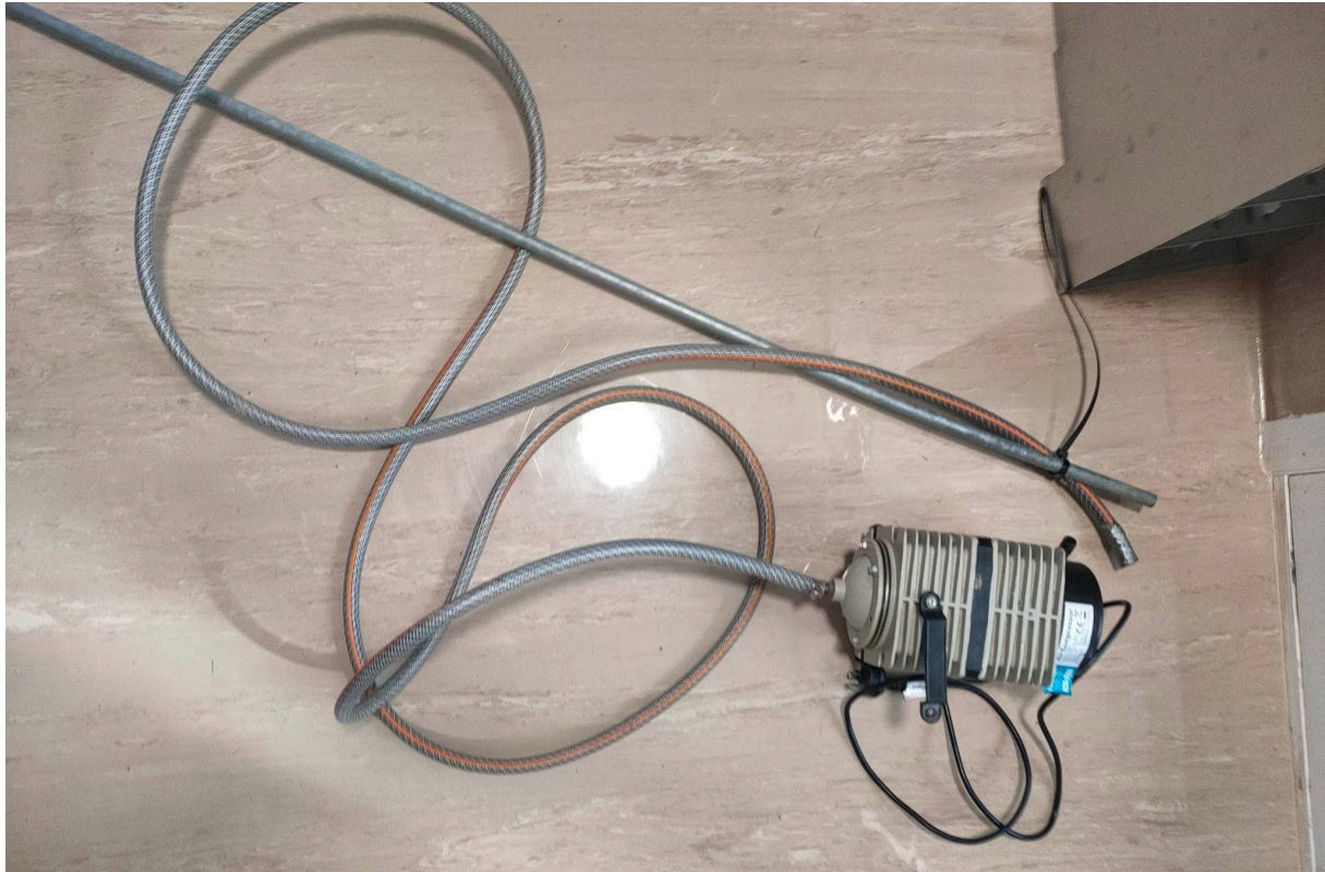
Figure 2. HAILEA air compressor attached to one end of a garden hose using a hose clamp (11-13 mm). The opposite end of the garden hose affixed to a steel rod using a zip tie.
