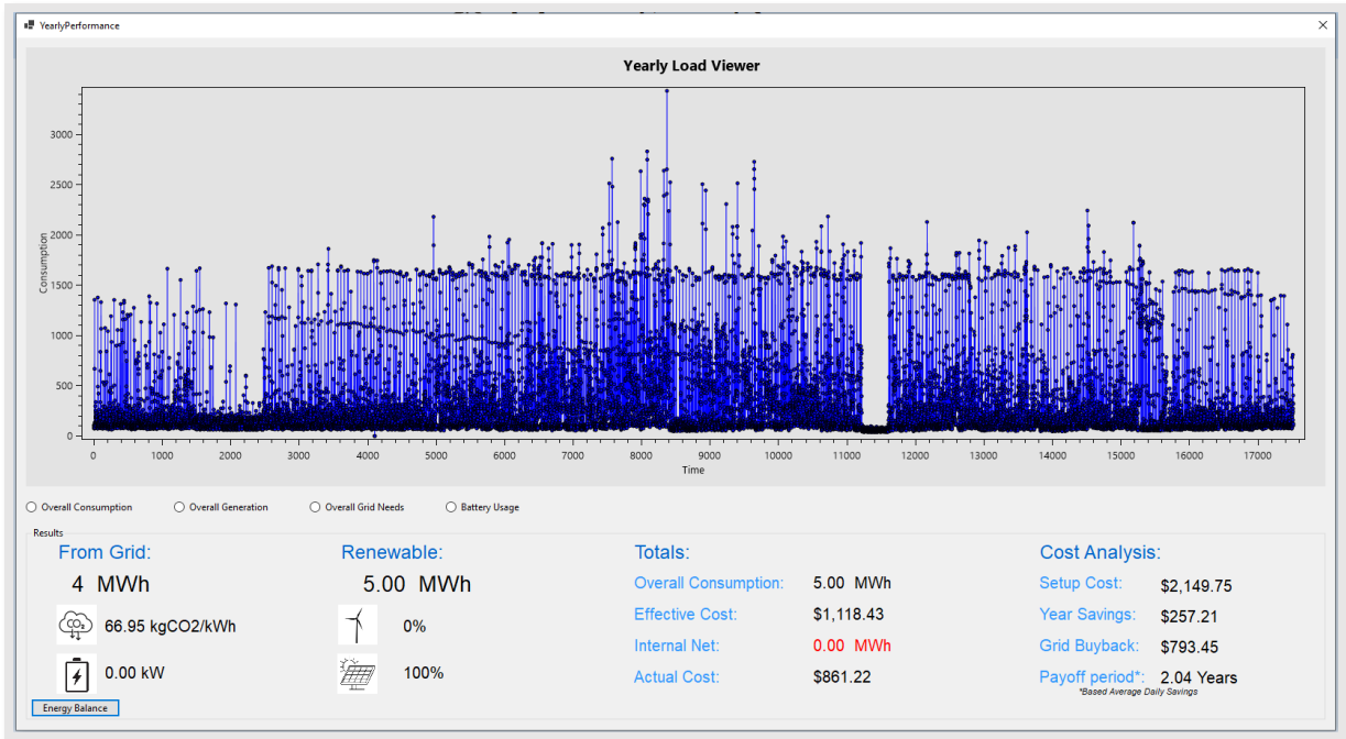
Figure 54 - Year report for case 1 after solar panels added to microgrid, costs being noteworthy
