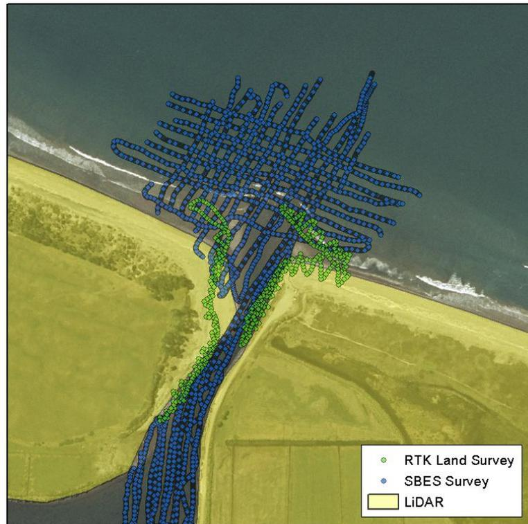
**Figure 4.2:** Map showing where the various survey methods were used, excluding the digitised hydrographic chart, which was used for the offshore region.
