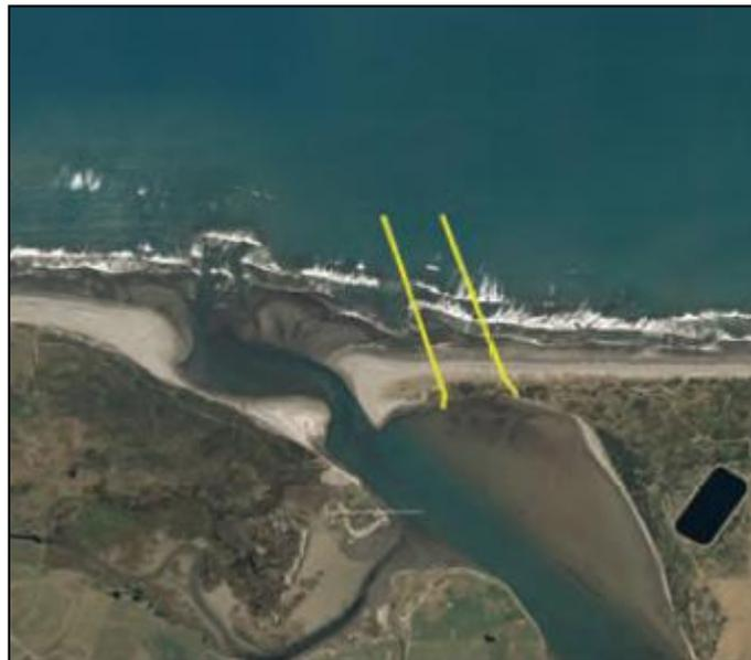
**Figure 3.13:** Aerial photograph showing the twin jetty structures that DHI (2008) concluded would provide the best navigation improvements, based on the required cost and flooding impacts (Modified from Pedersen *et al.*, 2008).
