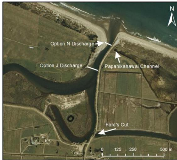
**Figure 7.2:** Map showing the two transects where discharge values were extracted from the model results for Option J and Option N.
