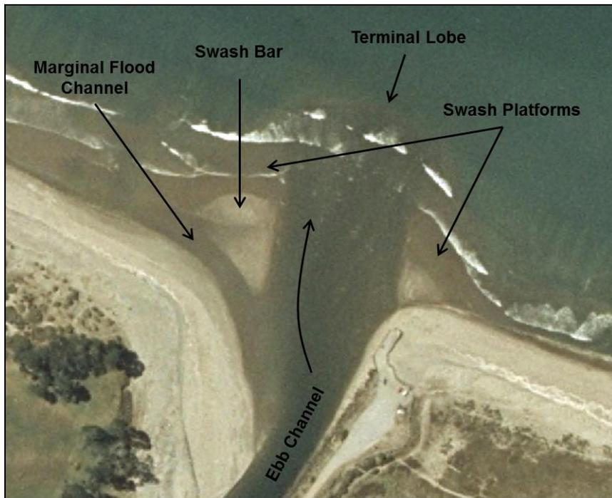
**Figure 3.2:** Aerial photograph showing the main features of the Te Tumu Cut ebb delta, in March 2008.
