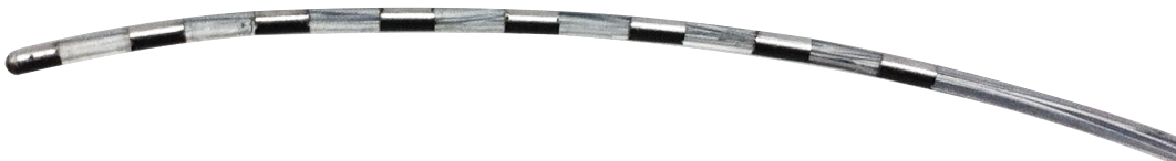
Figure 6.1: Distal end of an “Octrode” lead intended for SCS. Eight platinum electrodes, each 3 mm long and 1.3 mm in diameter, are separated by 4 mm insulating spacers.
