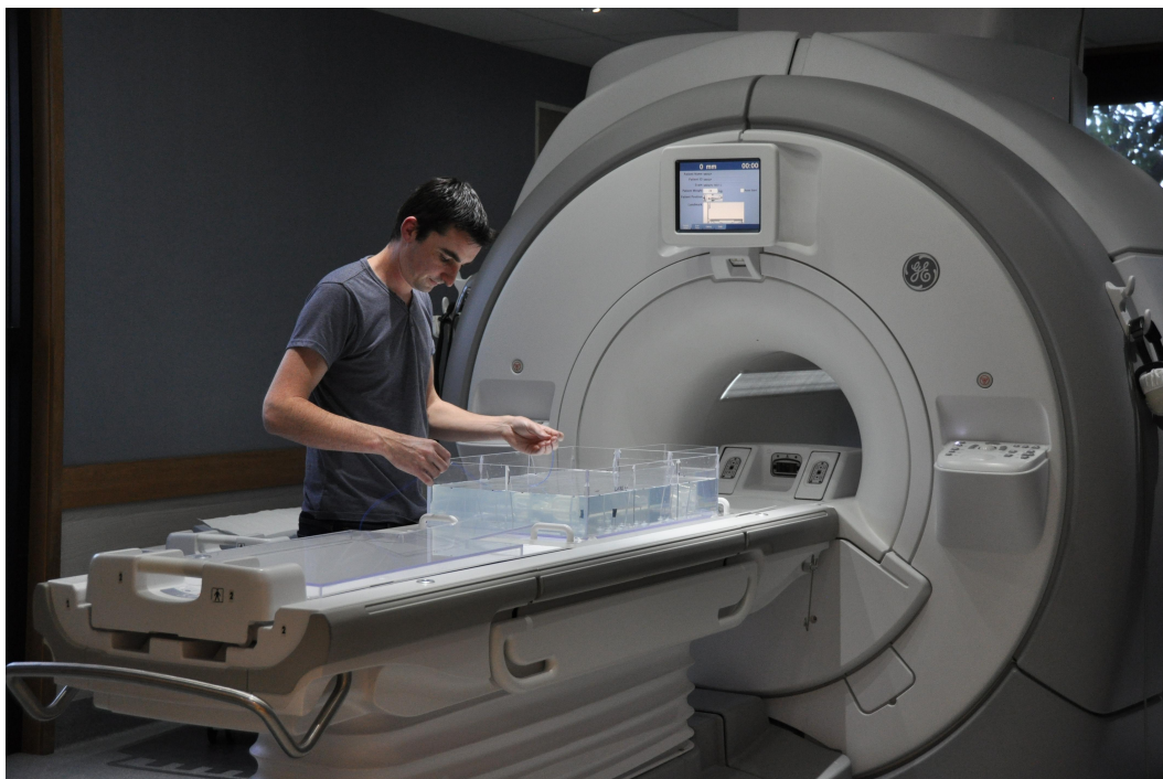
Figure 3.5: Clear acrylic phantom on the bed of the MRI machine with operator.
