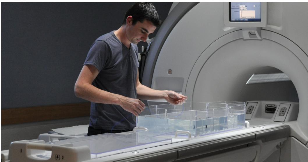
Figure 4.4: Clear acrylic phantom on the bed of the MRI machine with operator.
