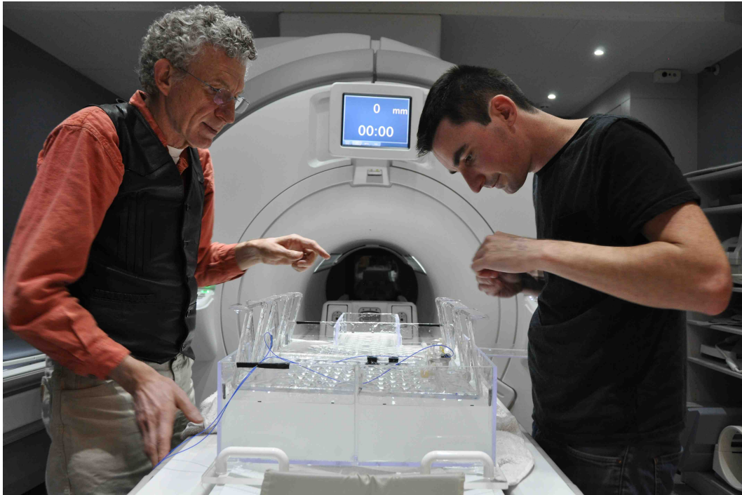
Figure 5.3: Operators preparing a wire sample for testing within a gelled saline phantom in a 3T MRI machine.
