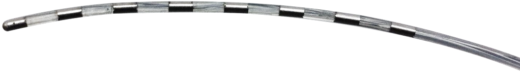
Figure 5.1: Distal end of a 62 cm SCS “Octrode lead”. Eight platinum electrodes, each 3 mm long and 1.3 mm in diameter, are separated by 4 mm insulating spacers. Electrode numbering starts from ‘1’ (left-most electrode) to ‘8’ (right-most electrode).
