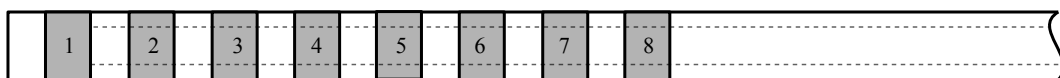
Figure 7.17: Model for simulating multi-electrode leads. Multiple lead filars are approximated by a single filar that extends and connects to each distal electrode. Insulation covers the filar and provides spacing between each electrode.
