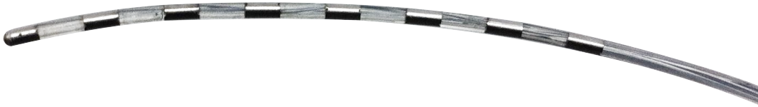
Figure 7.1: The distal end of an SCS lead with eight platinum electrodes. Each electrode is 3 mm in length, 1.3 mm in diameter, and spaced apart by 4 mm of insulation. Insulated platinum filars extend through the length of the lead to each individual electrode.
