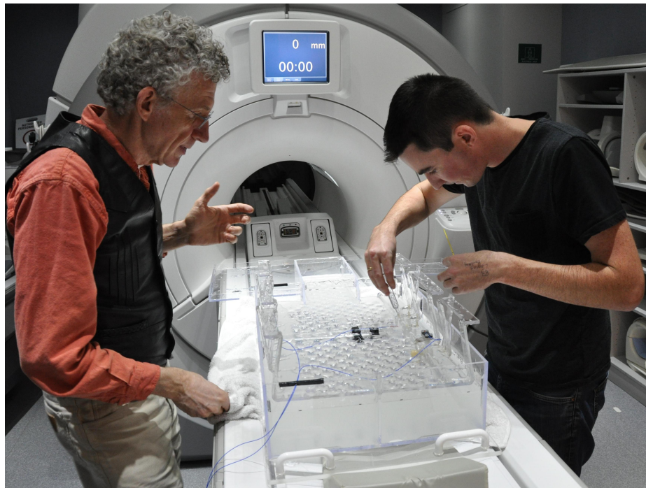
Figure 7.3: Operators position an implant lead inside of a gelled saline phantom on the bed of a 3T MRI machine. A GaAs-based fiber-optic temperature probe provides measurement of the distal electrode heating.
