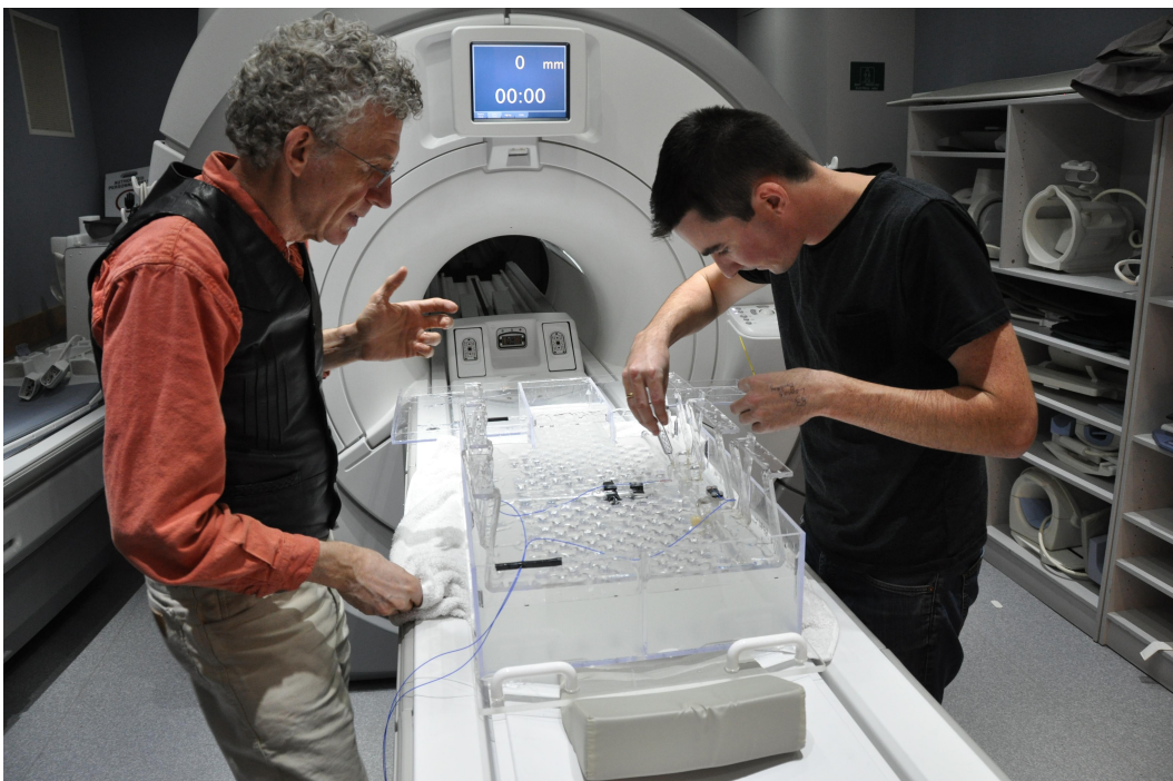
Figure 6.3: Clear acrylic phantom on the bed of the MRI machine with operators.
