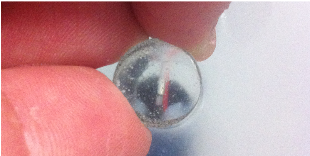
Figure 4.10: Alignment of the temperature probe with the distal electrode can be viewed through a solid acrylic bar with polished ends.
