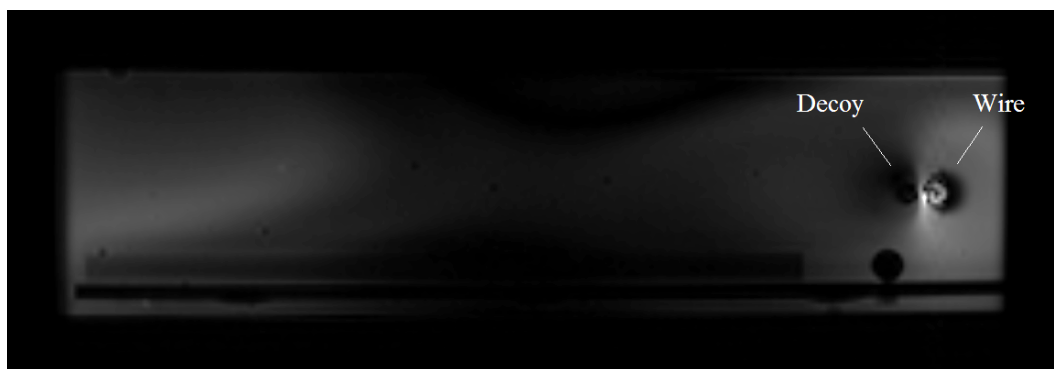
Figure 6.9: An MRI image showing the midpoint cross section of the phantom and decoy protected lead. Captured with a GE Healthcare Discovery MR750 3.0T machine [72].
