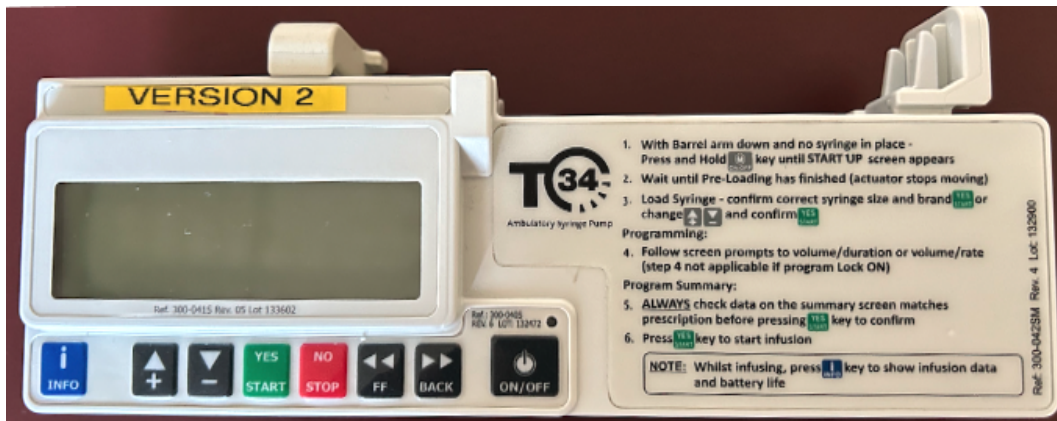
Figure 4.1: T34 infusion pump
