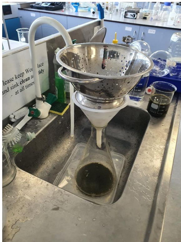
Figure 3-6. Straining of cow manure and distilled water solution to separate large solids
