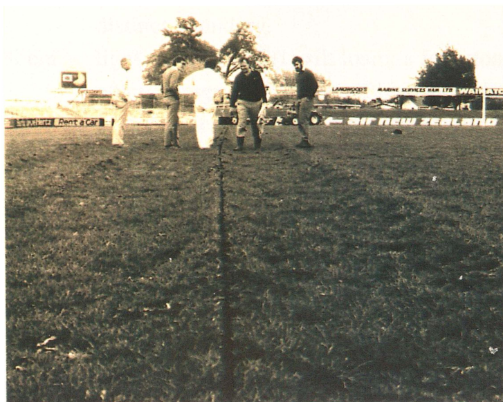
Figure 3.5.6 Rugby Park, October 1986. Subsoiled with prototype I (Figure 3.1.3). Note ground heave and slot opening.
