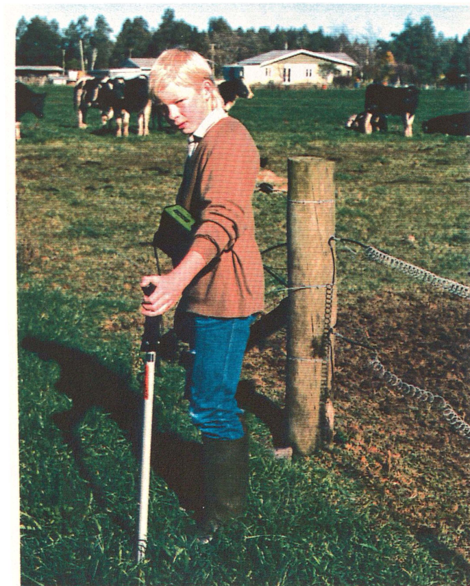
Figure 3.6.5 Pasture readings are made holding the probe stationary for 0.5 seconds.
