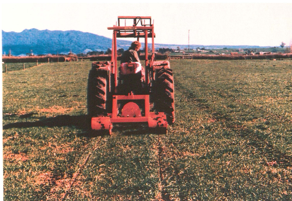
Figure 3.1.6 Pasture subsoiler prototype III, operating on Horotiu soil. Note reduced damage to pasture when compared with Figure 3.1.2
