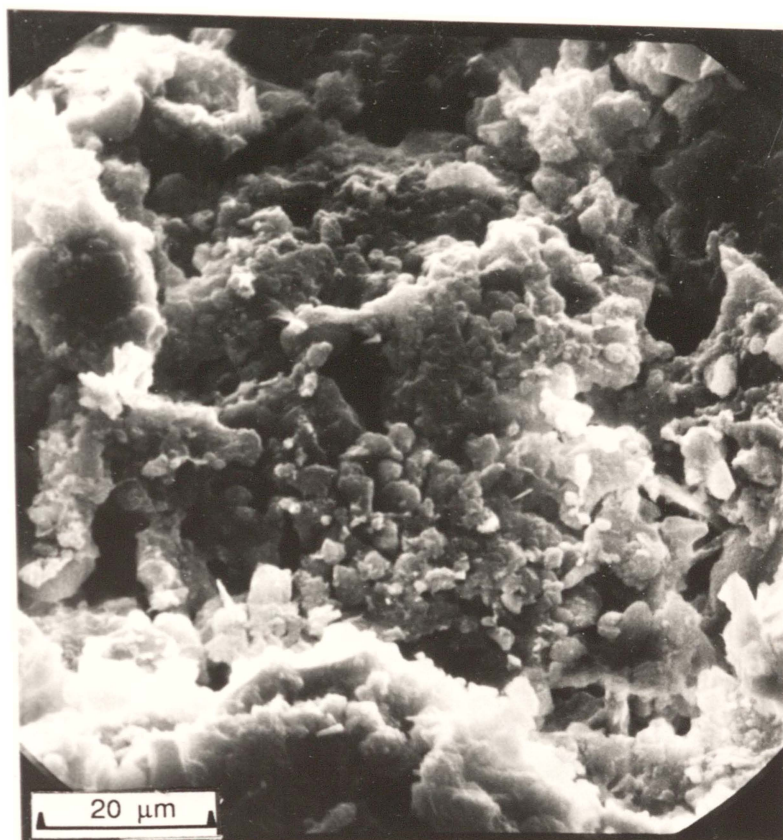
Figure 6.7.3 Rugby Park soil, high resolution SEM of A horizon aggregate (non-subsoiled)
