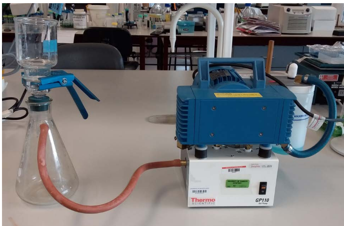
Figure 2. Vacuum system used to filter water sample through a glass-fibre filter.
