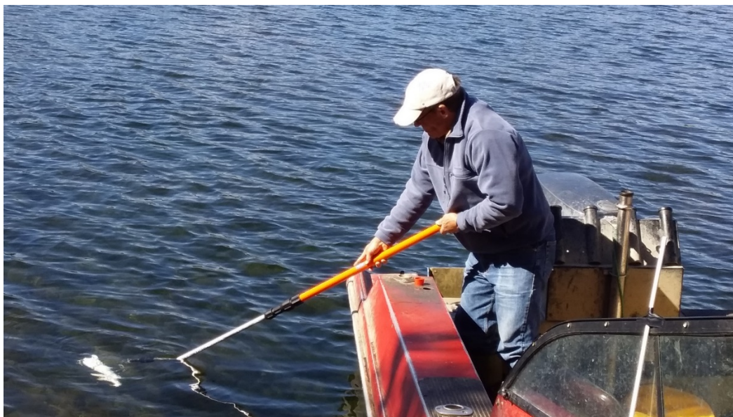
Figure 3. Water sample collection system, showing a 1-L plastic screw-top container mounted on a 3-m telescopic pole before rotation for filling.
