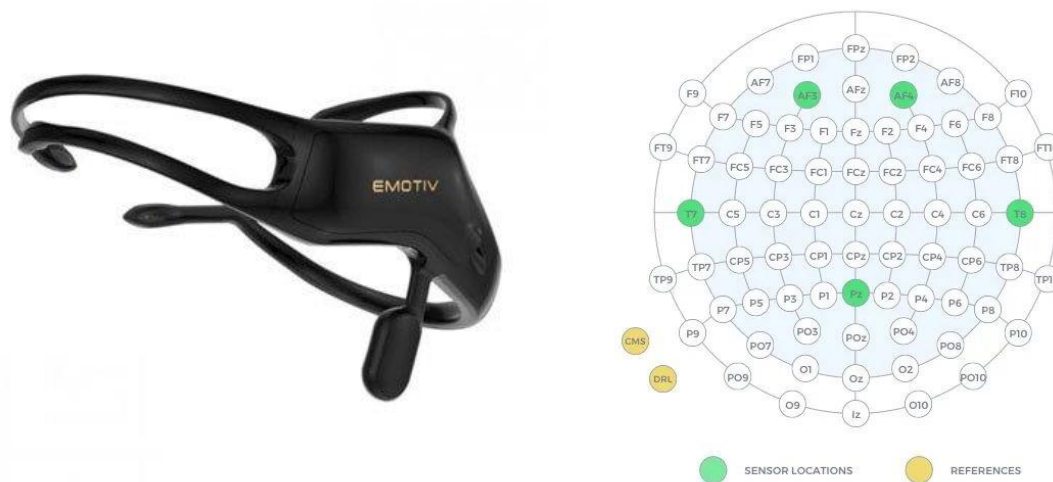
Figure 37: The Emotiv Insight sensor positions according to the International 10-20 sensor configuration[71]
