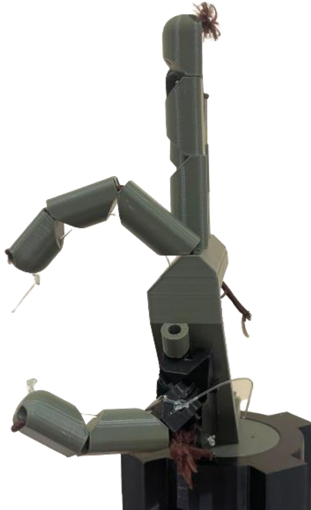
Figure 14: Fingers of "First" hand in partial flexion
