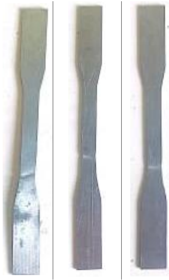
Figure A-2: Deformed shape of the coupons
