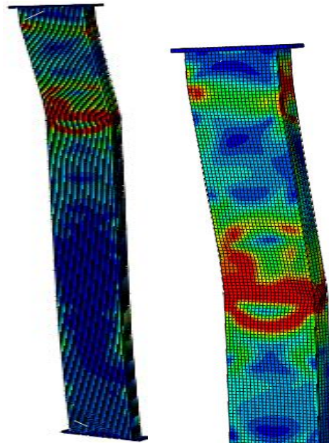
(d) Global buckling full view & detail view at one end
