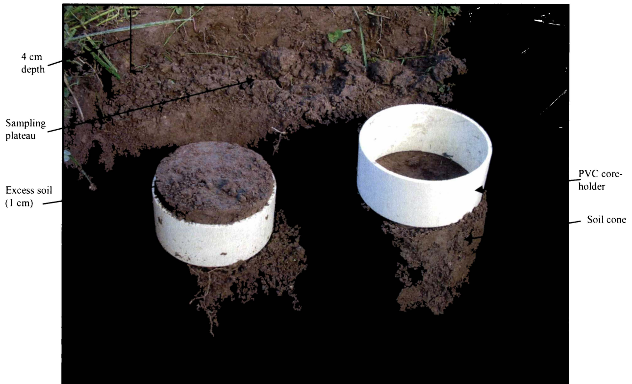
Figure 3.2 Porosity soil cores at the 5-10 cm soil depth before sampling (right) and immediately before removal (left).
