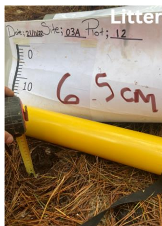
Figure 4.2. Measuring litter thickness at the centre of the DualEm-1 tube using a rigid measuring tape. Site (Mahurangi), Plot (12) and thickness were recorded.
