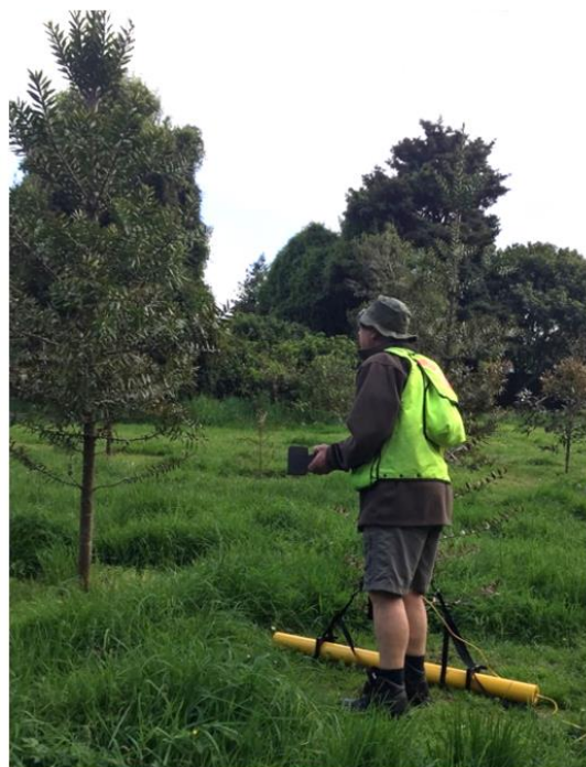
Figure 2.1. DualEm array with one transmitter (Tx) and receiver coils (Rx) pairs with windings oriented in horizontal co planer (HCP) and perpendicular co planer (PRP) (DualEm, 2014) (above). DualEm-1 in use at Scion’s Kauri nursery in Rotorua, New Zealand (below).
