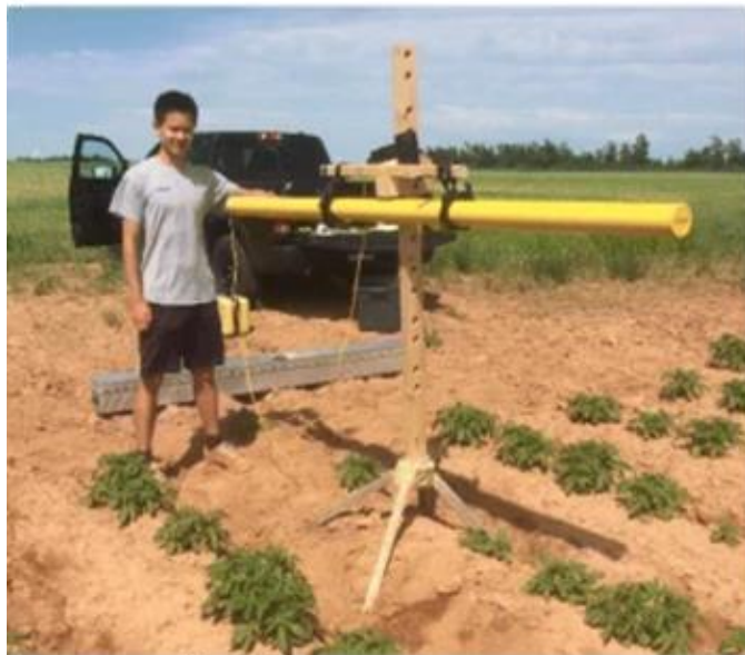
Figure 2.5. DualEm-2 Elevator for vertical electrical sounding (VES) (Tang et al., 2020).
