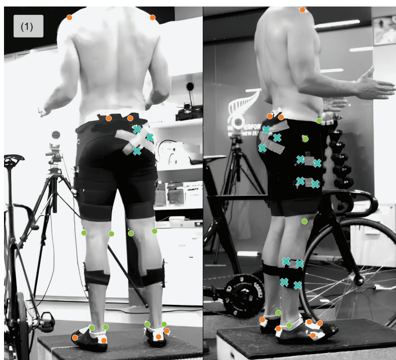
Figure 1. Position of the 45 retro-reflective markers (posterior and lateral views). The green circle markers were removed after the static trial; the clusters (crosses) and orange circle markers stayed on the participant during testing.
