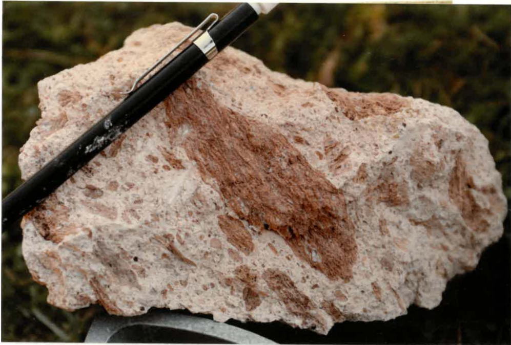
Fig. 3.15 Close up of strongly devitrified lapilli tuff. Note the well preserved lenticular, fibrous texture of the relic pumice. From the upper middle columnar jointed zone. Mamaku Ignimbrite, Scotts track.
