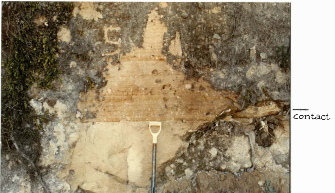
Fig. 3.37 Contact between two Waimakariri flows, note laminations in upper unit and complete absence in lower unit. Ruahihi Canal (U14/783727).
