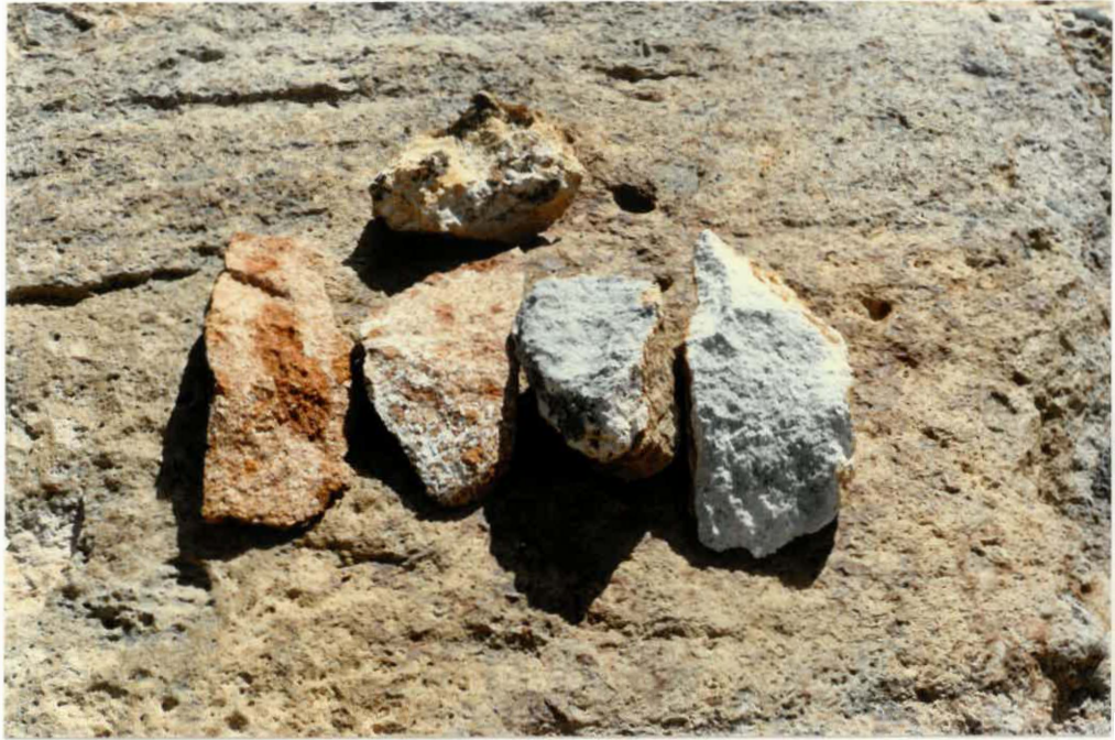
Fig. 3.38 Hand specimen examples of fresh (blue) and weathered (orange) mineralised Waimakariri Ignimbrite. Pumice is just visible in far left orange sample. Opuiaki River (U14/767695).
