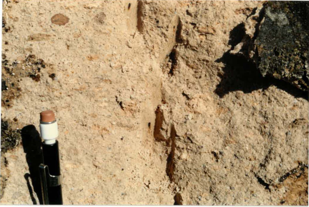
Fig. 3.14 Hand specimen of moderately welded, coarse and fine tuff, upper basal zone. Mamaku Ignimbrite, Scotts track (U14/777677).
