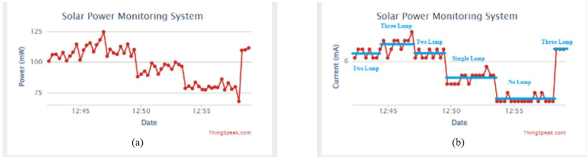
Figure 3.10: Performance Evaluation of the system under light bulb illumination, (a) voltage and (b) current.
