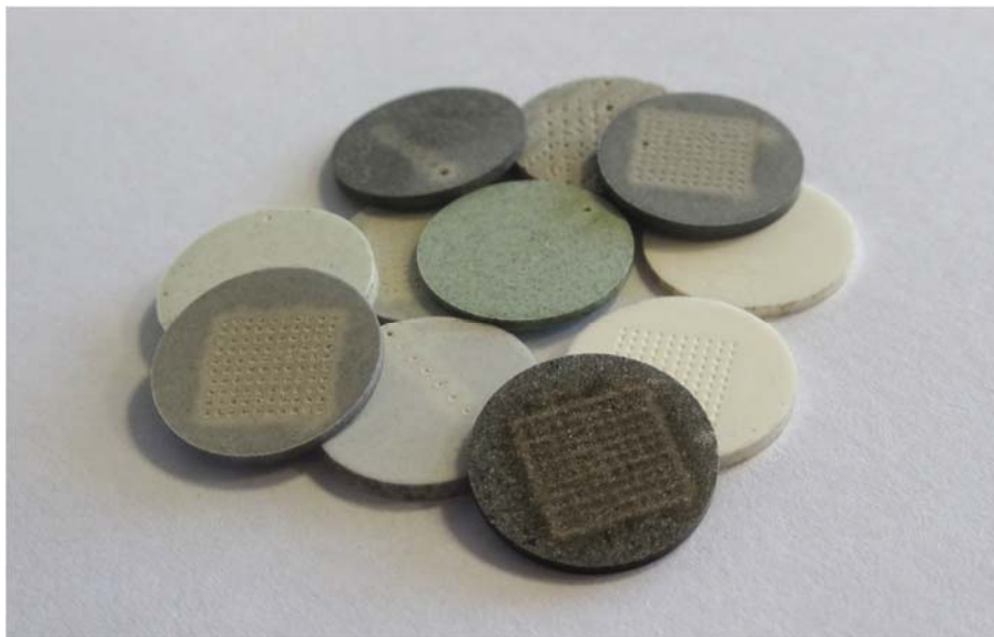
Figure 70: Photograph of pelletised samples for laser ablation. Dark pellets contain metal nanoparticles, white pellets are blanks, and green pellets are blanks doped with cobalt acetylacetonate. Note the different patterns of dots on the samples' surfaces, produced by laser-induced breakdown.
