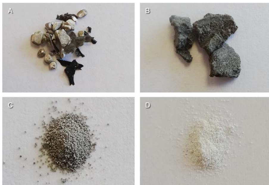
Figure 93: Photographs of four catalysts materials prepared by three different immobilisation methods. The four pictures correspond to: a) Rh-PVA/HAp prepared by rotary evaporation, b) Rh-PVA/MCC prepared by acetone precipitation, c) Rh-PVA/Al 2 O 3 prepared by adsorption, and d) Rh-PVP/Al 2 O 3 prepared by adsorption.
