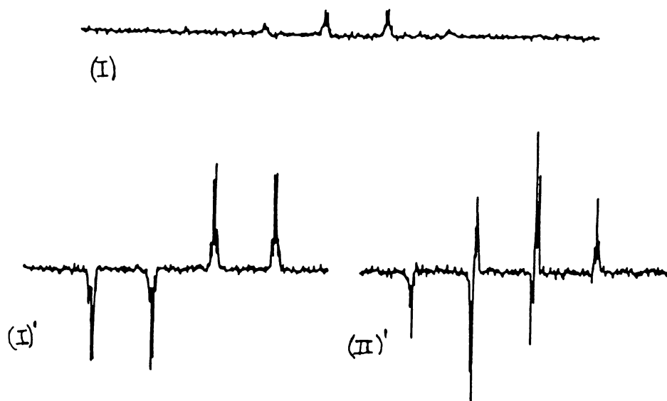
FIG. 3.5 Coupled ^{73}\text{Ge} INEPT via ^1\text{J} and ^2\text{J} coupling; both under the same experimental conditions as the unenhanced coupled experiment (NON). The spectra were from a sample of \text{GeMe}_3 for which ^1\text{J}(\text{Ge},\text{H}) = -94.3 \pm 1.1 Hz and ^2\text{J}(\text{Ge},\text{H}) = 3.48 \pm 1.1 Hz. (I) (I)' using NON and ^1\text{J} INEPT, respec., with 482 scans, 1000 Hz, 8K (II)' using ^2\text{J} INEPT with 482 scans, 1000 Hz, 4K.
