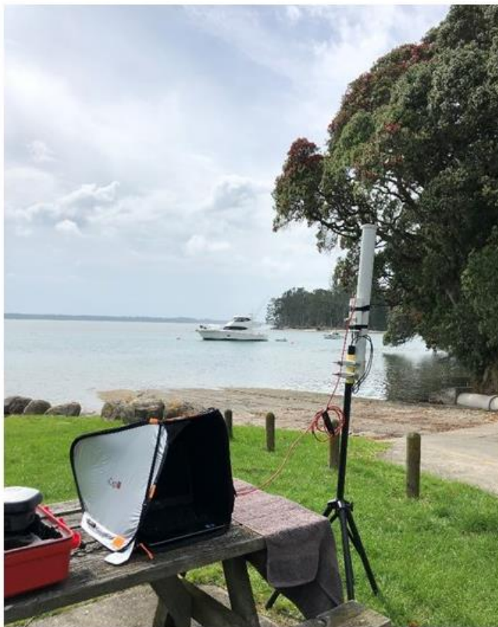
Figure 2.4. JetYak base station set up with connection to field laptop inside Icap.
