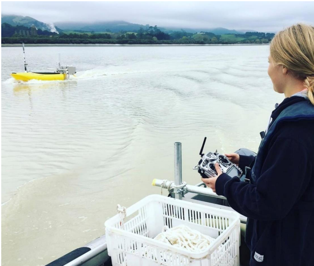
Figure 4.4. JetYak being remote controlled during the survey from research vessel through the Waihou River in the Firth of Thames.
