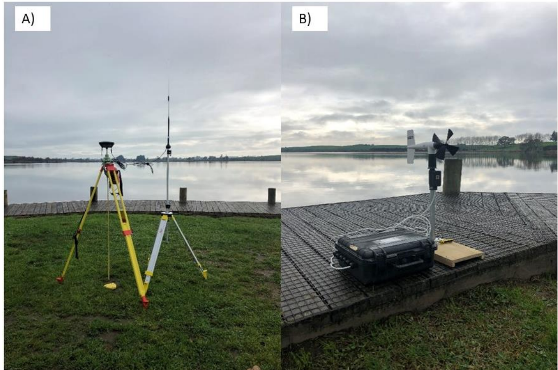
Figure 2.6. A) Base Station set-up for RTK GPS at Lake Ngaroto. B) Wind Sensor set-up at Lake Ngaroto.
