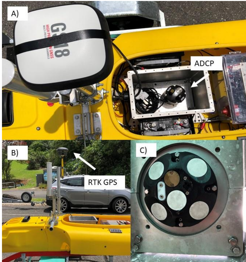
Figure 3.3. A) RTK GPS and ADCP set up on board JetYak with ADCP mounted in the sea chest. B) Side view of JetYak with RTK GPS set up. C) ADCP mounted downwards facing into sea chest.
