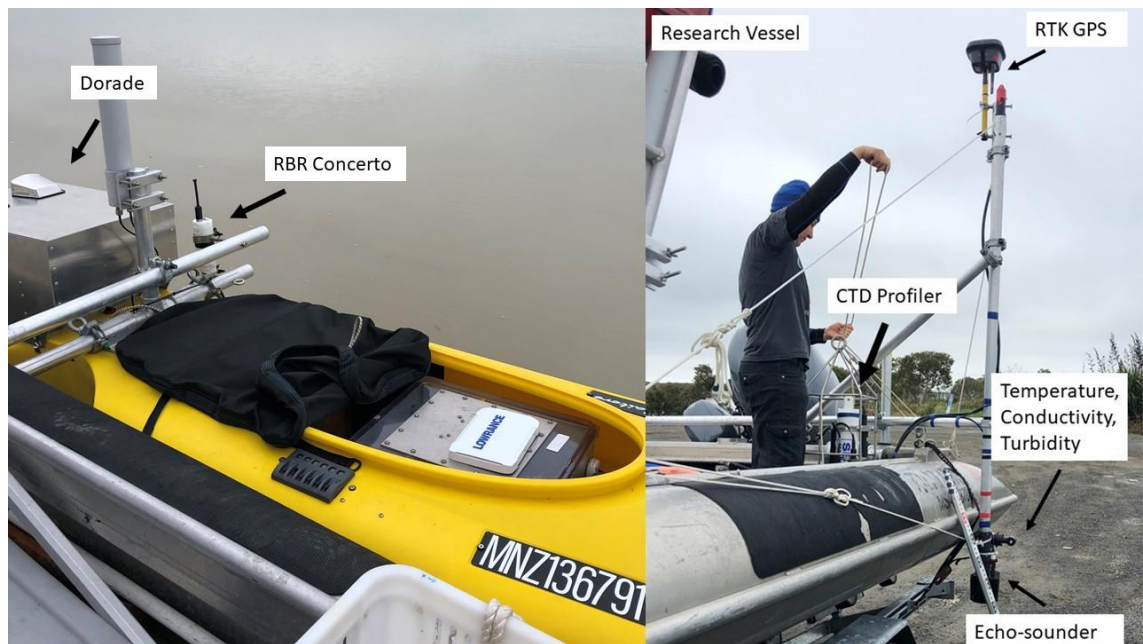
Figure 4.2. JetYak and Research vessel instrument and dorade set-up.
