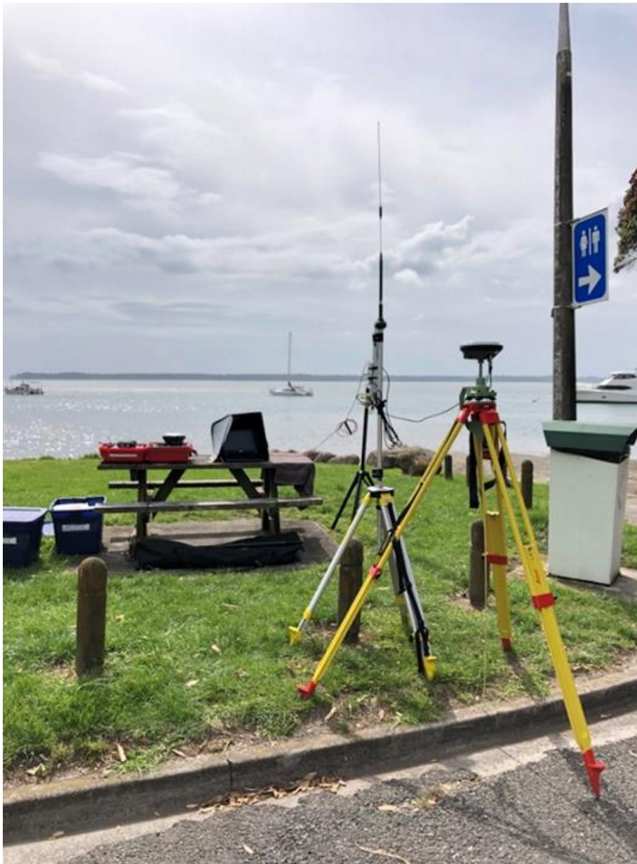
Figure 3.2. RTK GPS Base station and JetYak laptop set-up at Tanners point.
