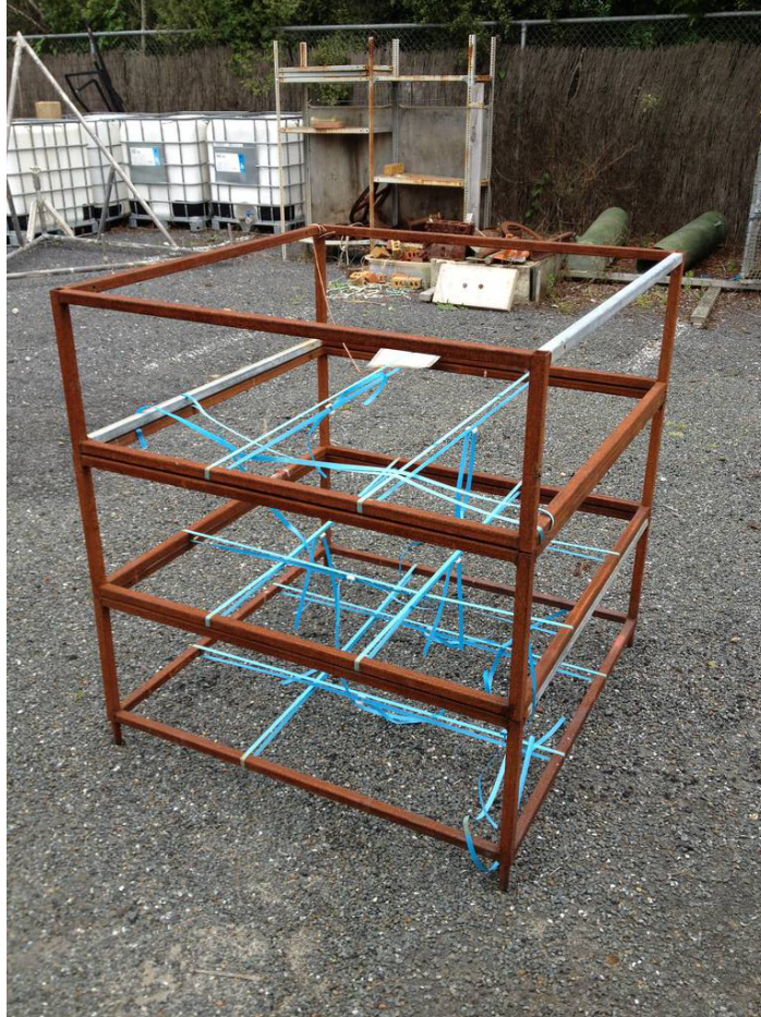
Figure A.1: The first cage constructed to collect drifting macrophytes (three separate but stackable layers, steel bars, welded).
