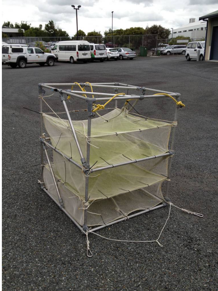
Figure A.2: The second cage constructed to collect drifting macrophytes (one rigid outer frame with space for one to four vertical layers of nets, aluminium tubes, modular screw-fixed fittings/joints).
