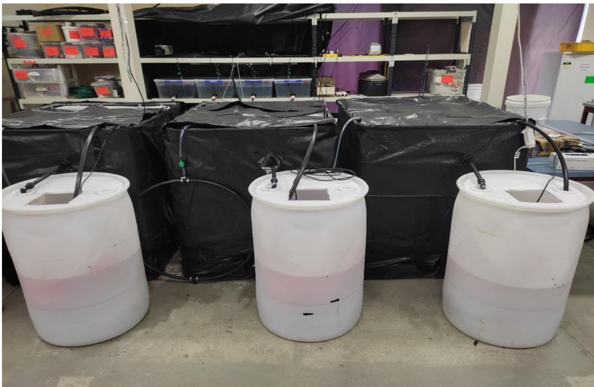
Figure 2.2: The experimental RAS system, consisting of three separate recirculating tanks with dedicated biofiltration units.
