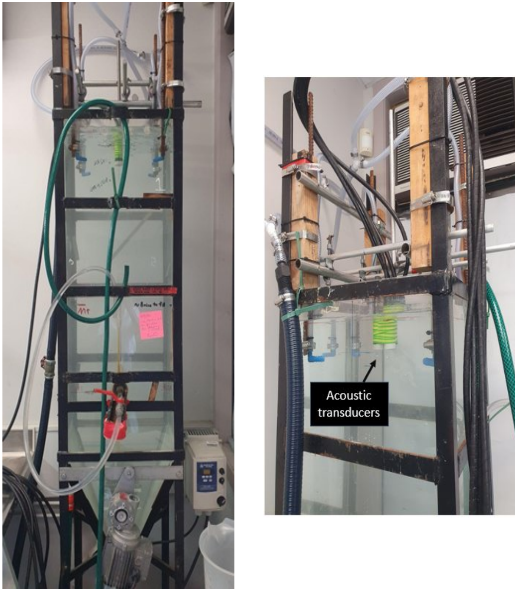
Figure 3.3: Laboratory experimental set-up of tank with linked ABS device for ballotini bead suspension experiments: a) front view with single 3MHz transducer mounted (B) b) side view with grouping of 1, 2, 2.5 and 4 MHz transducers mounted (A).
