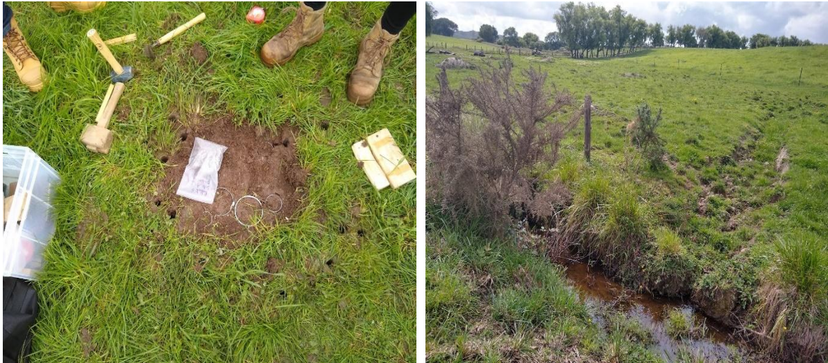
Figure 3-16: Field sampling at the study site: (Left) Soil core extraction using a hand auger for laboratory analysis of physical and chemical properties; (Right) Drainage pathway where water samples were collected to assess suspended sediment load, nutrient content and potential estrogen transport in surface runoff.
