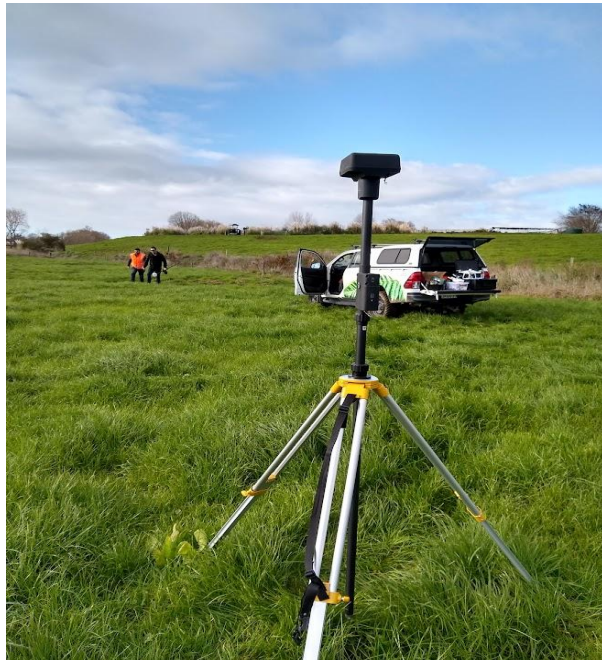
Figure 3-19: Drone-based survey for high-resolution DEM generation at the dairy farm site. The DJI drone was deployed (top left) and launched from a designated landing pad (top right) to capture aerial imagery of the site. The ground control setup (bottom left) was established for accurate georeferencing, and a GNSS receiver (bottom right) was used for additional spatial calibration.
