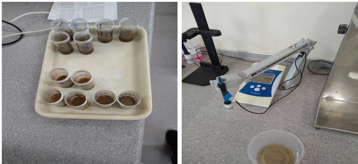
Figure 3-18: Soil pH measurement setup. (Left) Prepared soil suspensions (1:2.5 soil-to-water ratio) equilibrating before measurement. (Right) pH probe immersed in a soil solution for reading using a calibrated pH meter
