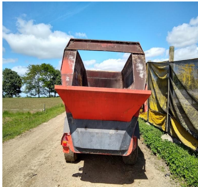
Figure 3-11: Effluent solid spreader used on dairy farm for applying solid dairy effluent onto pasture
