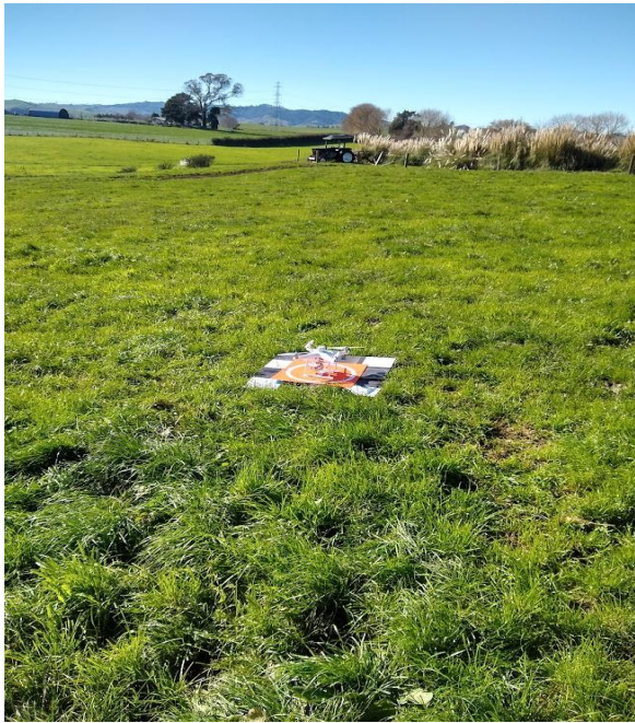
Figure 3-19: Drone-based survey for high-resolution DEM generation at the dairy farm site. The DJI drone was deployed (top left) and launched from a designated landing pad (top right) to capture aerial imagery of the site. The ground control setup (bottom left) was established for accurate georeferencing, and a GNSS receiver (bottom right) was used for additional spatial calibration.
