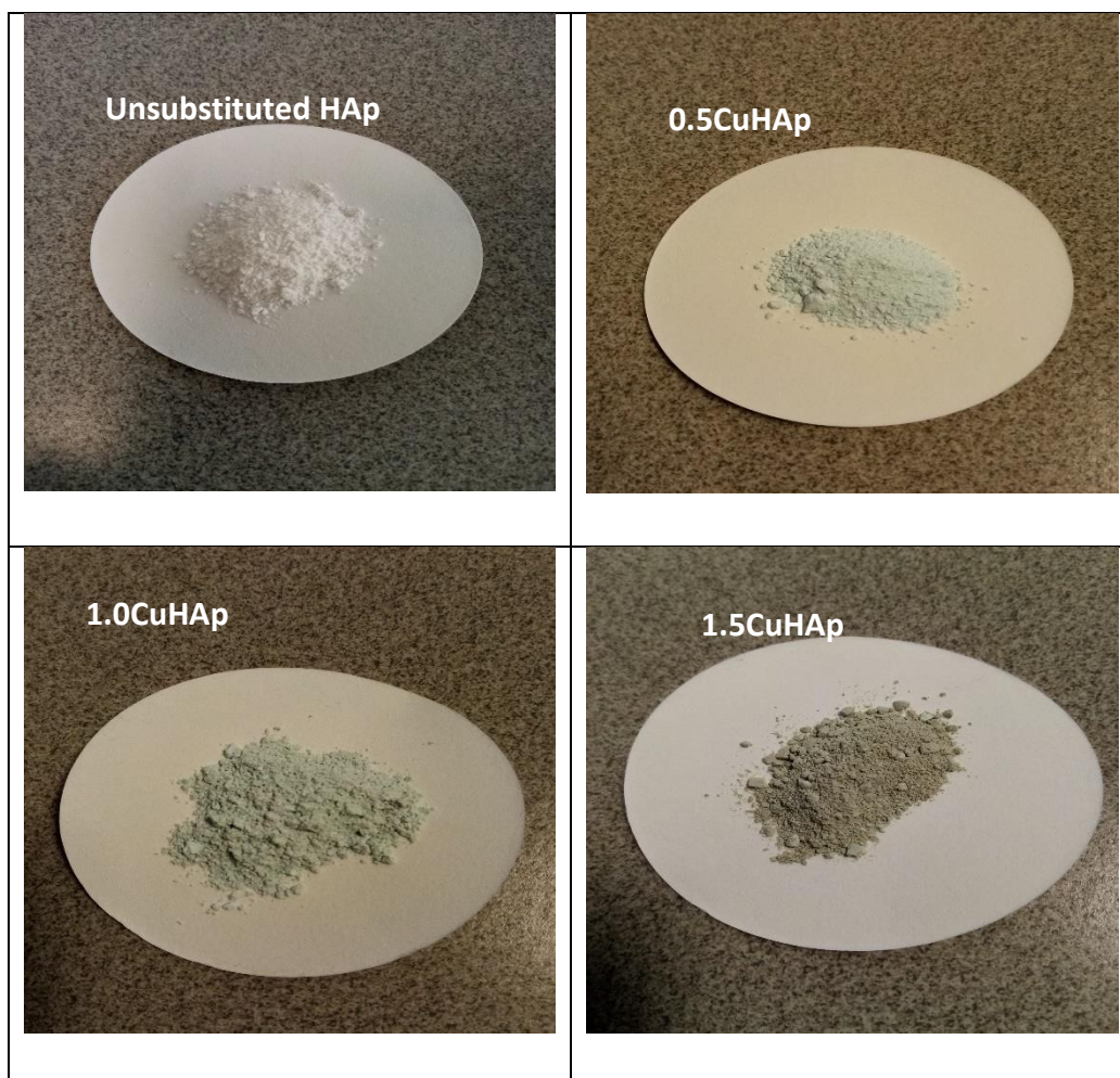
Figure 5-9: Colours of the non-sintered CuHAp materials containing different levels of \text{Cu}^{2+} ion substitution as prepared by the hydrolysis of \text{MCP}/\text{Ca}(\text{OH})_2
