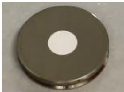
Figure 3-5 Sample holder as used in powder X-ray diffraction and the way powdered samples were packed into the holder with an even surface.
