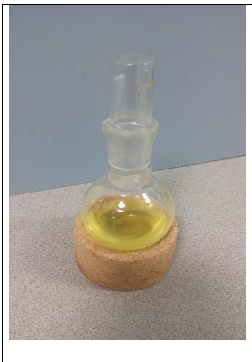
Figure 7-1: NbCl 5 solution that resulted from dissolving Nb 2 O 5 in 12 M HCl and heated at 200 °C with reflux for 10 hours.
