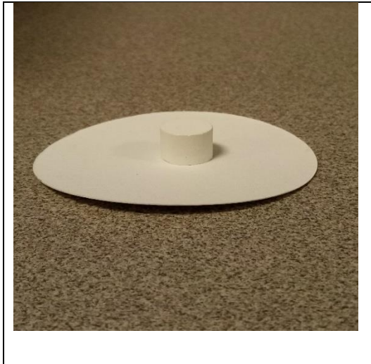
Figure 3-6: The cylindrical specimens of (10 mm) height and (11.2 mm) in diameter fabricated from prepared HAp material produced by the hydrolysis method.
