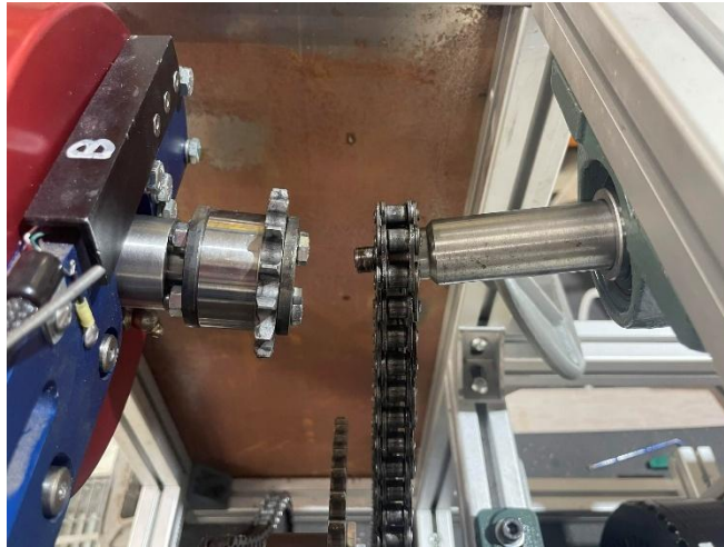
Figure 74. Testing Rig Shaft Failure
