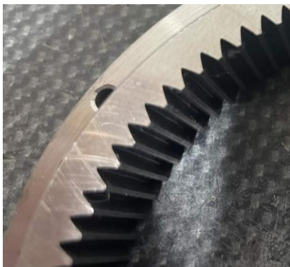
Figure 79. Ring Gear Striations
