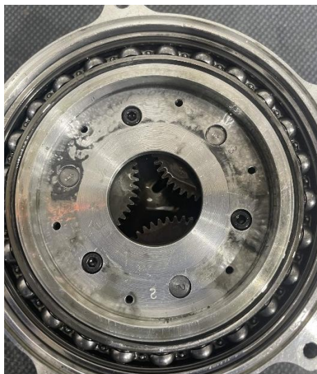
Figure 77. Residue Around Shaft 1
