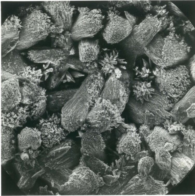
Figure 4.6 Weathered recrystallized calcite. Both the large calcite rhombs and the smaller recrystallized calcite show pitting and weathering. This is a typical view of the surface of a calcite pseudomorph. Sample C918 (80x) (by Dr. C. Beltz)
