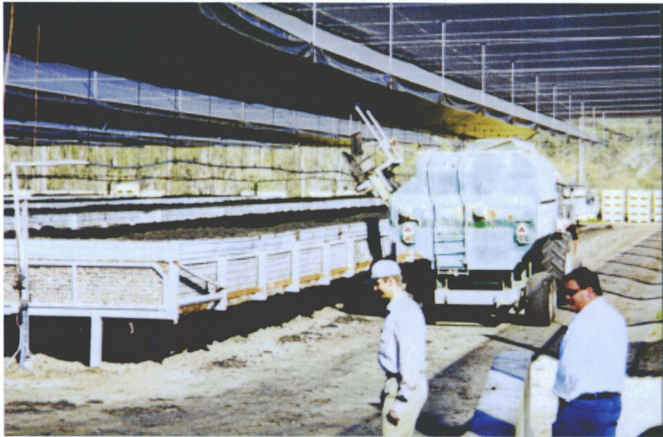
Figure 6: Continuous flow raised beds for large-scale vermicomposting operation (Vermitech Pty. Ltd., Redland, Qld, Australia).
