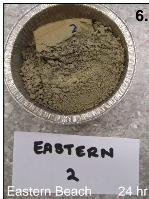
Figure 5.4: Various stages of the modified jar slake test. The I_j' value is written at the top right corner of each photograph.
