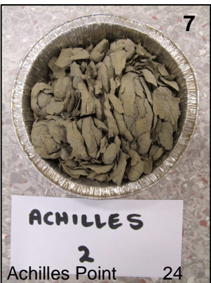
Figure 5.4: Various stages of the modified jar slake test. The I_j' value is written at the top right corner of each photograph.
