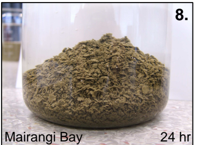
Figure 5.4: Various stages of the modified jar slake test. The I_j' value is written at the top right corner of each photograph.
