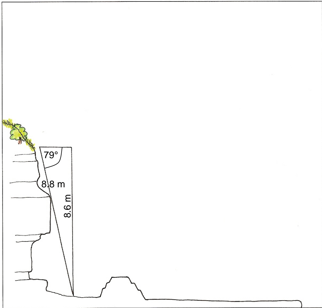
Figure 4.17: Photographs and sketch of the described Mairangi Bay cliff section. A: Cliff face with lower encased sewer pipe (red bracket) which acts as a sea wall. B: Dark iron-stained sandstone joint faces; thin siltstone bed is between dashed lines. C: Cliff profile and shore platform (extent is marked by white arrow); sewer pipe is marked by red line. D: Sketch of bedding and shore platform characteristics.
