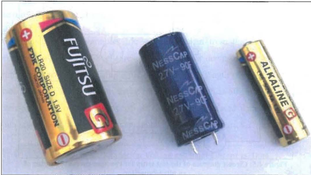
Figure 4.4: Photo of a 90 farad, 2.7 volt ultracapacitor next to a D-size battery and an AA-size battery
