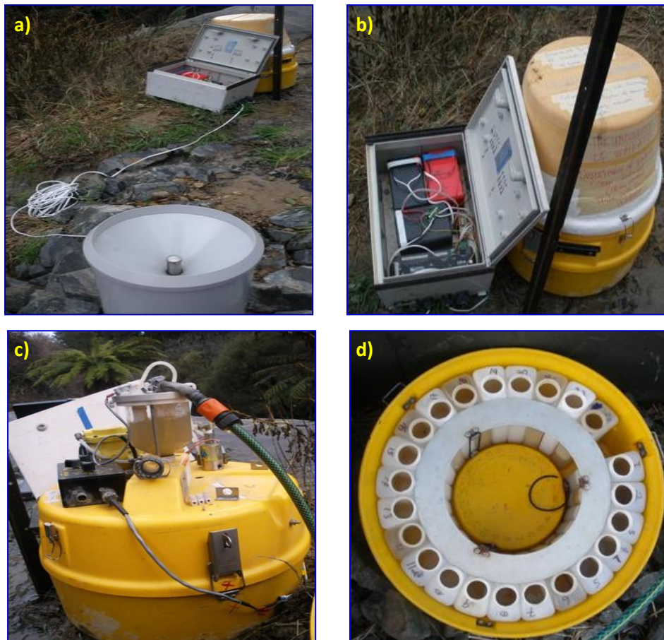
Figure 4.5 Inflow sample collection at sediment retention ponds using autowater sampler; a) Rain gauge connected to Campbell Scientific CR10x data logger; b) Campbell Scientific CR10x data logger which is connected to autowater sampler; c) The autowater sampler which operated on 12-volt wet cell battery; d) Twenty four polypropylene sampling bottles.
