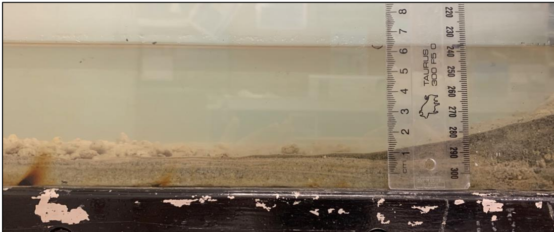
Figure 4.16 – Photograph of layers deposited by all six experimental runs.
