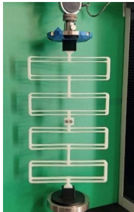
Figure 4: Compression test setup.
