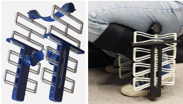
Figure 14: Exoskeleton system: Compli-Knee assembly (left) and engaged proof of concept on left leg (right).
