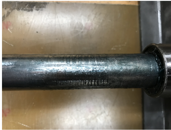
Figure 4.17: Damaged caster king pin.
