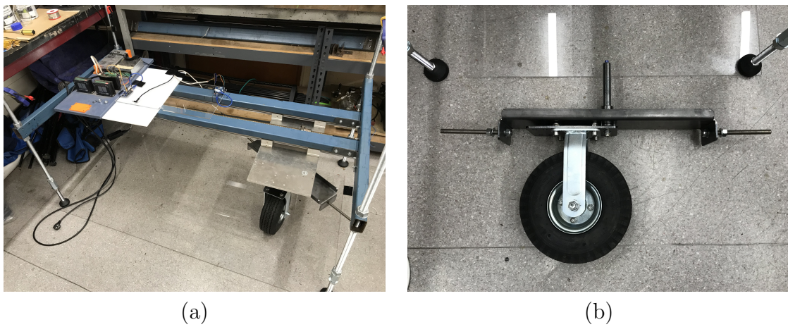
Figure 4.3: Caster experiment photos, full rig (a) and caster assembly (b).
